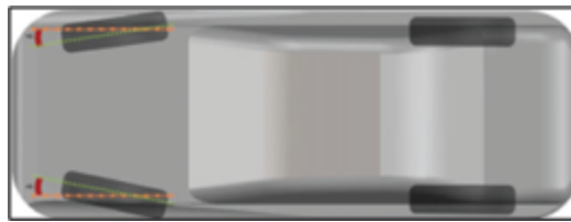
Figure 46. Toe Angle in a Vehicle Suspension System (Goodarzi and Khajepour 2017)
