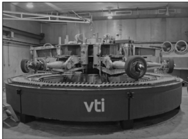
Figure 43. VTI Road Simulator (Gustafsson et al. 2012)
