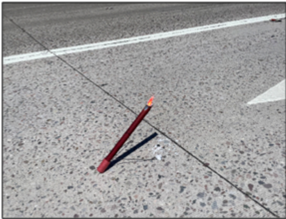
Figure 34. Burning Flares in the HOV Lane During Sampling
