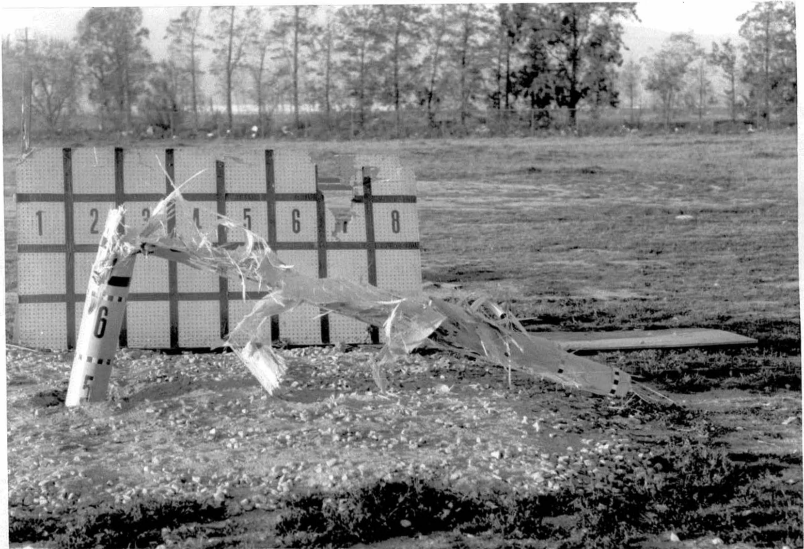
Figure 62. Closeup of pole break away, posttest, test no. 4.
