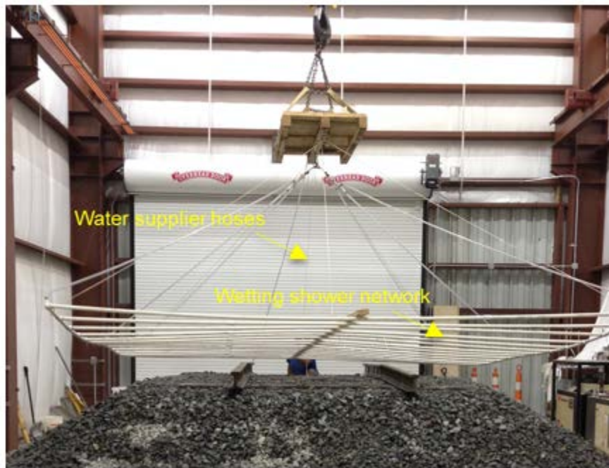
Figure 6. Apparatus Used to Wet the Models. Water Was Supplied to a Grid of Perforated PVC Pipe Via a Network of Feeder Hoses
