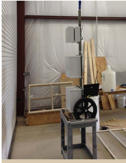
Figure 15. Calibrating the RABIT by Collecting Data at Various Distances from a Planar Reflector
