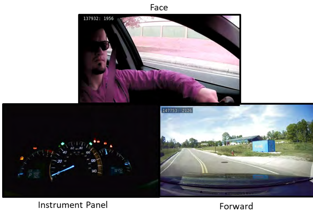
Figure 1. VTTI DAS camera views: face, instrument panel, and forward.
