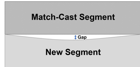
Bowing distortion caused by the heat of hydration in the new segment.
