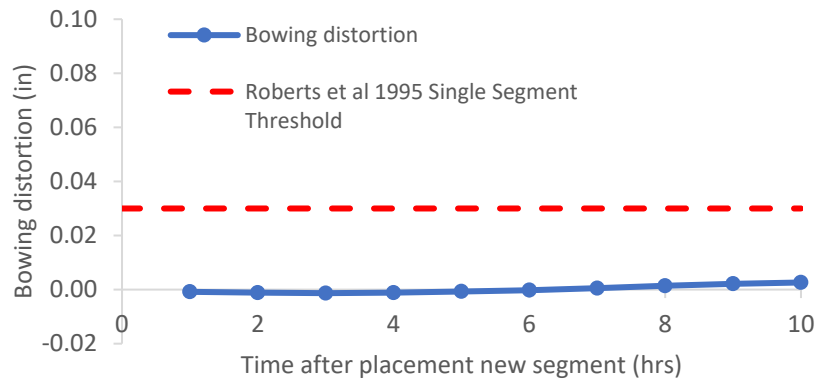
Figure B-434: Simulation 145 - Bowing distortion progression of match-cast segment from time of placement of new segment to 10 hours
