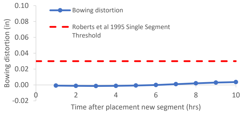
Figure B-422: Simulation 141 - Bowing distortion progression of match-cast segment from time of placement of new segment to 10 hours
