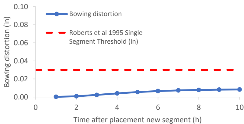
Figure B-29: Simulation 10 - Bowing distortion progression of match-cast segment from time of placement of new segment to 10 hours
