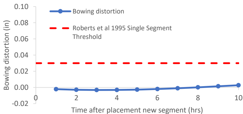
Figure B-389: Simulation 130 - Bowing distortion progression of match-cast segment from time of placement of new segment to 10 hours
