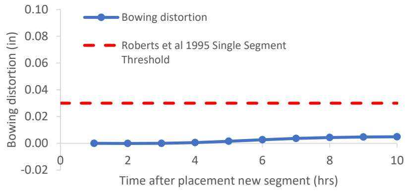
Figure B-326: Simulation 109 - Bowing distortion progression of match-cast segment from time of placement of new segment to 10 hours
