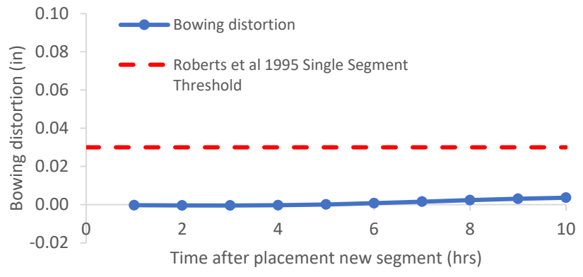
Figure B-374: Simulation 125 - Bowing distortion progression of match-cast segment from time of placement of new segment to 10 hours
