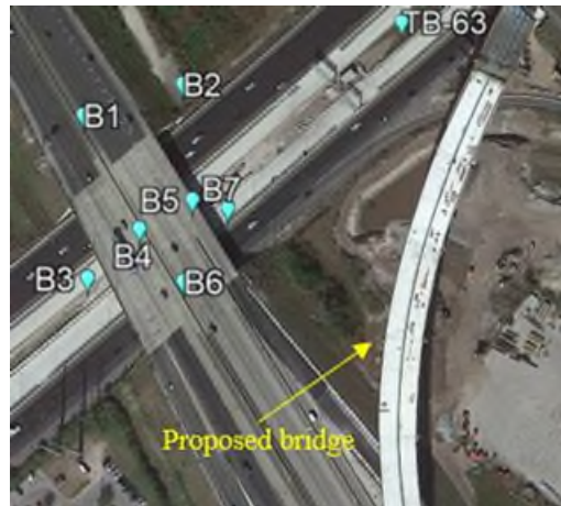
Figure 3-17. Location of soil borings relative to the construction site at Site D (Map data © 2021 Google).
