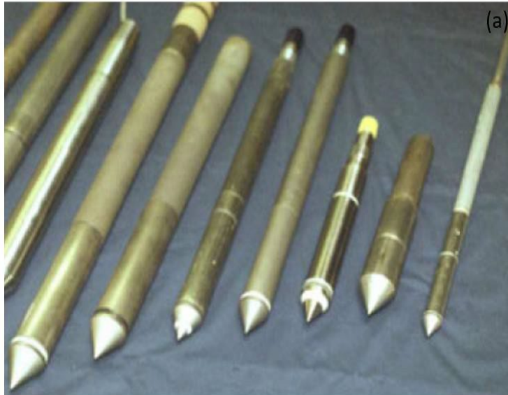
A. Several of the GT-acquired cone penetrometers in varying sizes and sensor configurations from Mayne (2007b)
