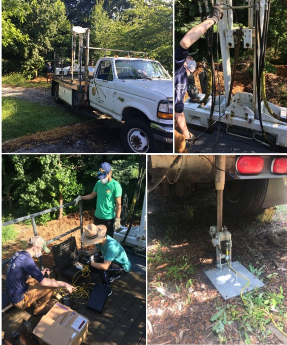
Figure 13. Photos of GT field crew using the Vertek HT cone penetrometer system.
