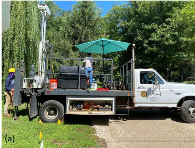
A. Georgia Tech CPT rig in operation in the State of Illinois
