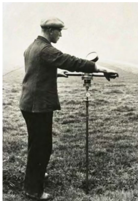
A. Dutch cone penetrometer field operation
