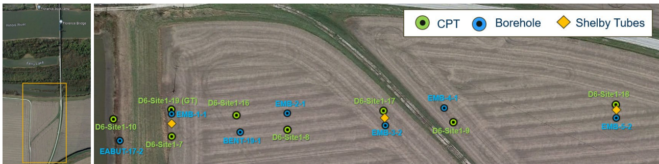
Figure 165. Photo of locations of Florence CPT soundings and borings for Shelby tube samples.
