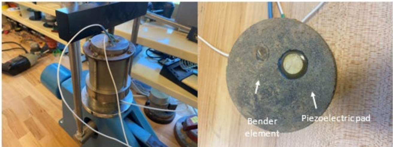
Figure 182. Laboratory shear wave measurement Photos: consolidation cell with wave measurement settling on an oedometer (left); inside view of the top cap showing bender element for shear wave velocity measurement. This setup can also measure compressive wave through piezoelectric pads (right).
