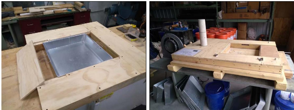
Figure 34. Wind erosion test apparatus during fabrication and final construction
