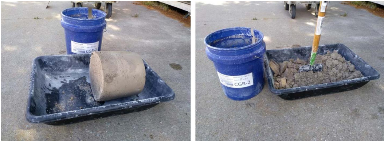
Figure 30. Consolidation of CGR slurry after storage for extended period of time (left) and CGR solids broken up with a garden hoe (right)
