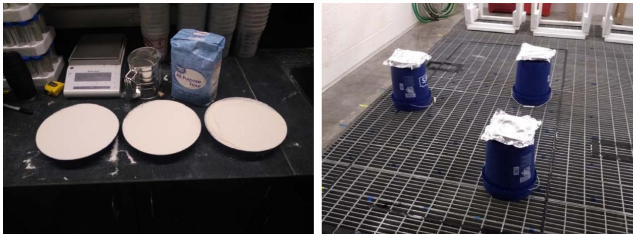
Figure 19. Raindrop particle size distribution test (flour test)
