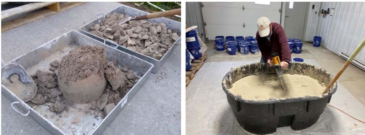
Figure 4. Typical CGR cakes (left) and CGR slurry mixing process (right)
