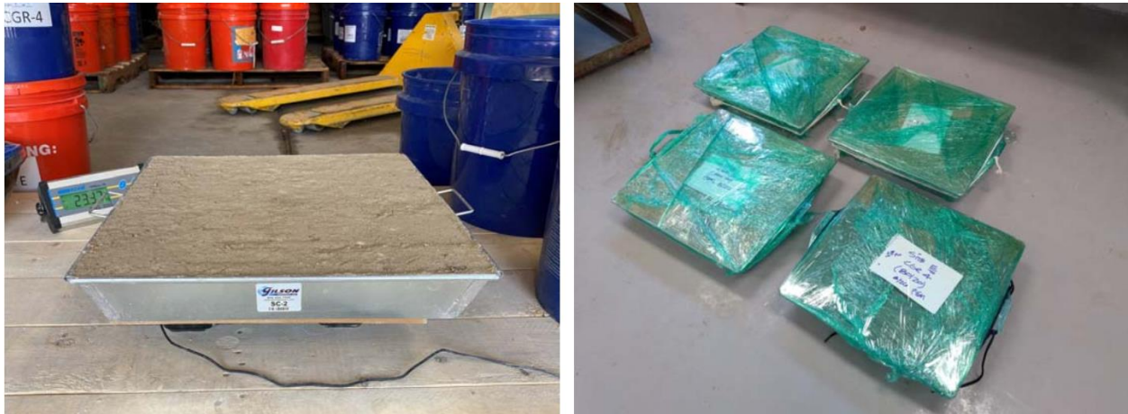
Figure 38. Weighing of compacted soil (left) and curing of (sealed) compaction soil forms (right)
