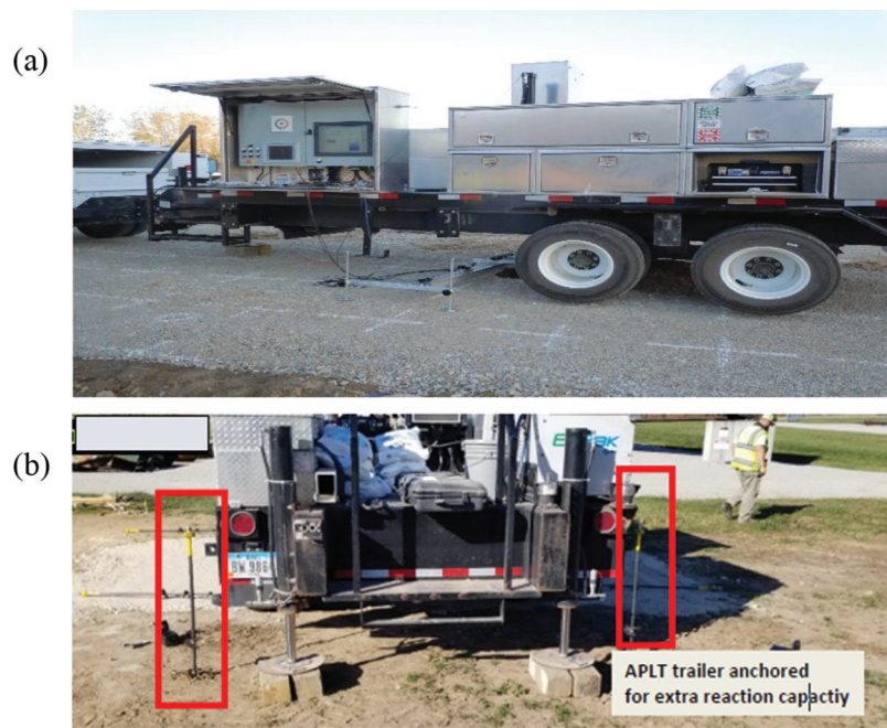
Figure 3.17 APLT static test setup: (a) without anchors, and (b) with anchors (adapted from Ingios, 2021).
