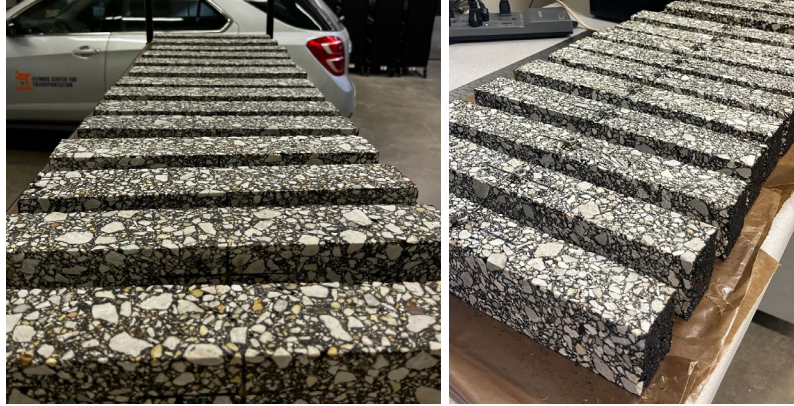
Figure 20. Photos. Examples of compacted and sawed beams.
