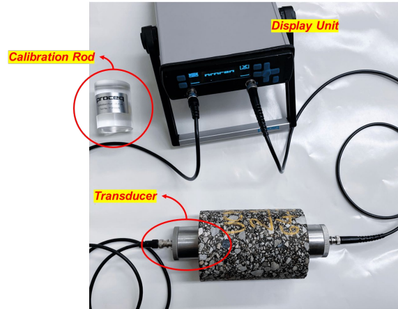
Figure 16. Photo. UPV device.
