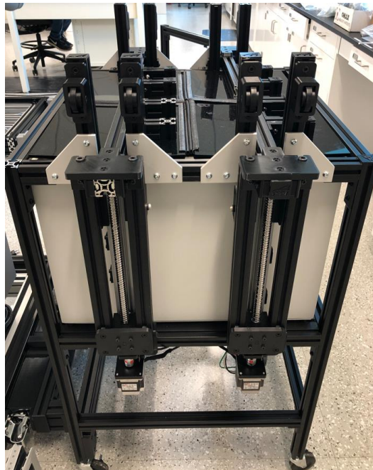
Figure 7. Specimen Conditioning Unit for IDEAL-CT (or IDEAL-RT)
