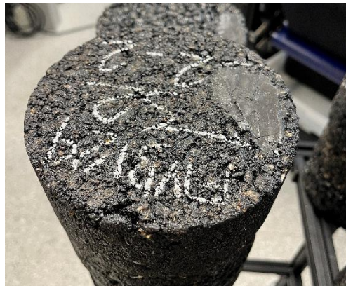
Figure 12. RFID Tag on Asphalt Specimen
