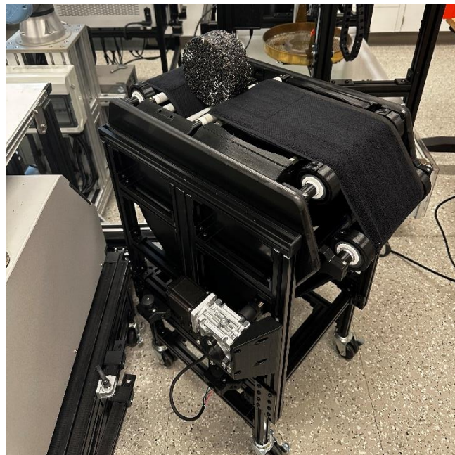
Figure 6. Saturated Surface Dry Component
