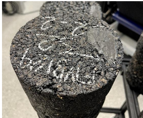
Figure 12. RFID Tag on Asphalt Specimen
