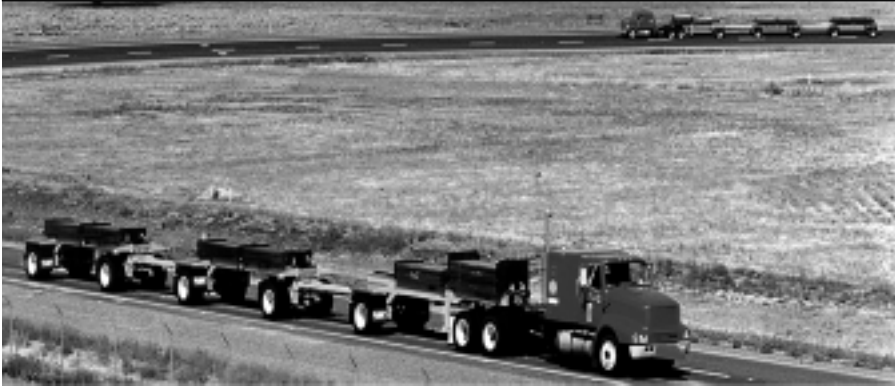
Figure 1. WesTrack Driverless Vehicles (Gross Vehicle Weight 670 kN [152,000 lb])
