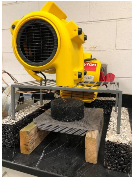
Figure 16. Rapid Cooling Unit with Two Fans.
