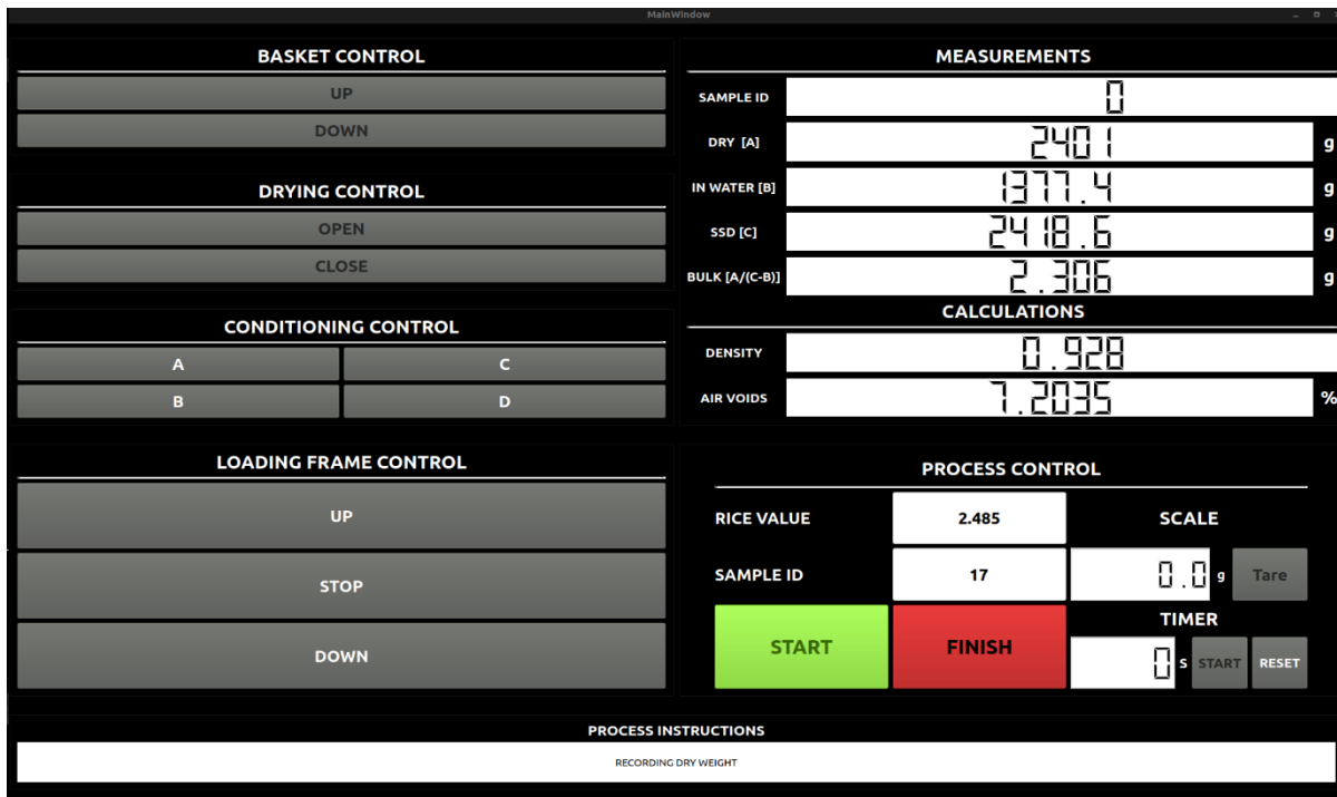
Figure 20. Computer Control Interface for Specimen Air Void Measurement.
