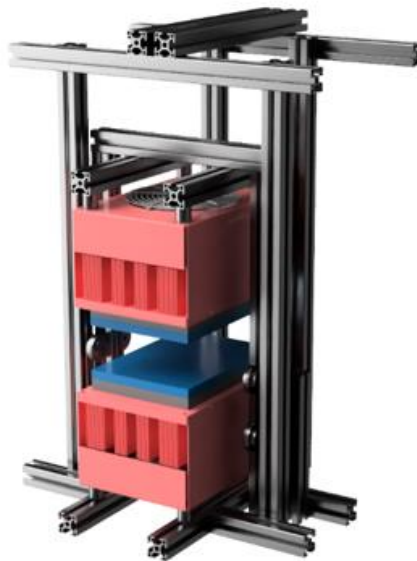
Figure 14. Rapid Cooling Unit.
