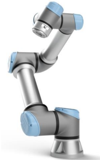
Figure 23. Robotic Arm: UR5e.
