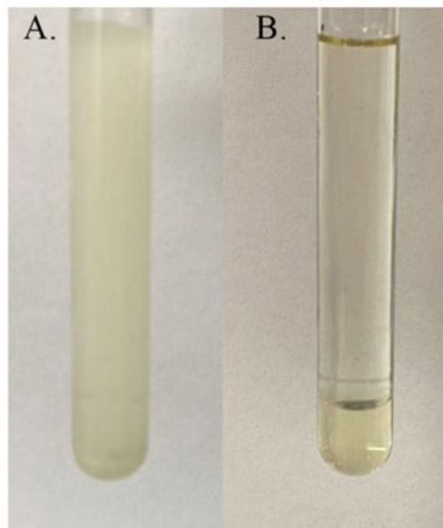
Figure 2.17 Emulsified fuel (10E5W) sample immediately a) after ultrasonication, and b) after phase separation [18].
