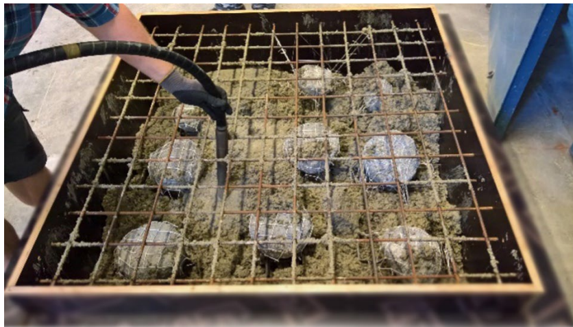
Figure 24. Photo. Specimen fabrication with preinserted honeycombs.
