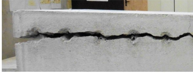
Figure 2. Photo. Total split of the specimen due to improper borehole design.
