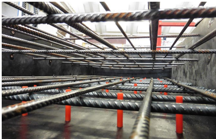
Figure 4. Photo. Using PVC cylinders (red) to create boreholes in a concrete specimen, saving drilling effort.
