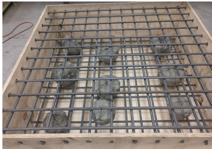
Figure 26. Photo. Specimen with preinserted honeycombs by Research Laboratory B.
