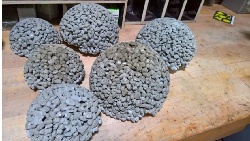
Figure 23. Photo. Prefabricated honeycombs in different sizes.
