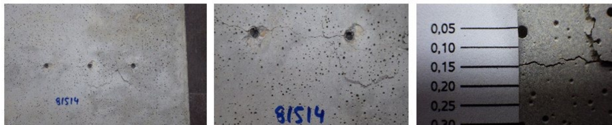
Figure 9. Photos. Crack width measurement 3 d after filling the expandable material.
