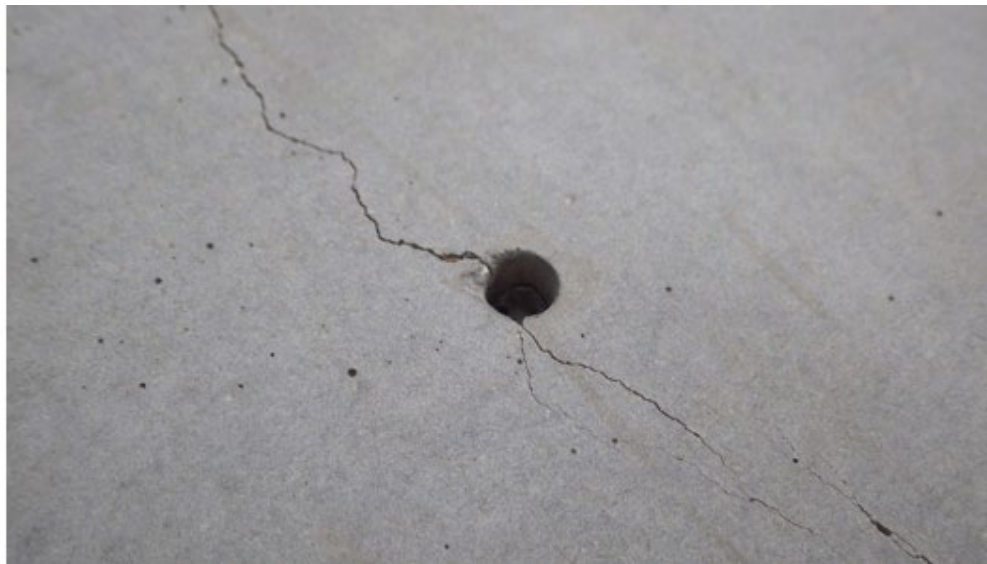
Figure 7. Photo. Cracks created without concrete spalling by filling expandable material in only to 10-cm below the surface level.
