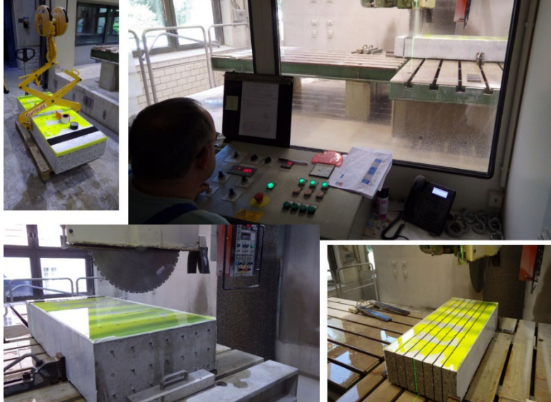
Figure 10. Photos. Destructive testing to evaluate the internal cracks by cutting the specimen.
