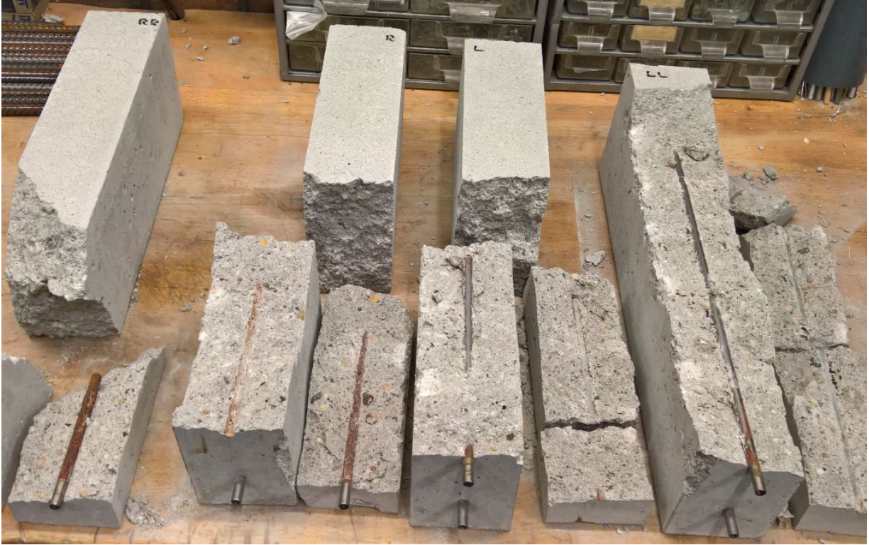
Figure 32. Photo. Destructive evaluation of concrete specimens to measure material loss.
