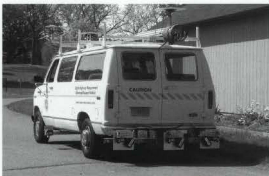
The Digital Highway Measurement van combines a variety of instruments on a single vehicle to provide accurate, efficient analysis of roadway geometry and pavement conditions.
