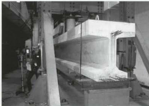
A load is placed on an I-shaped beam made of self-consolidating concrete to determine adequate development length between the concrete and the steel strands shown protruding from the end of the beam.
