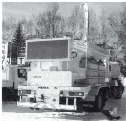
Snowplows with dynamic message signs and additional lighting attached to the back of the vehicle, such as the one shown above, increase visibility at the rear of the vehicle.
