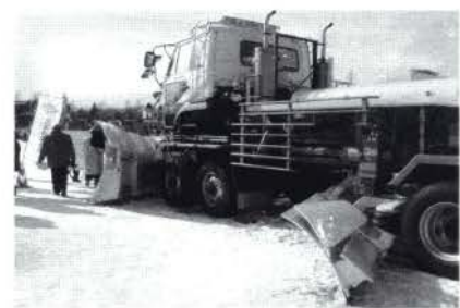
A snowplow with a cab-over design, twin front axles, and a plow located under the body of the vehicle is shown above.
