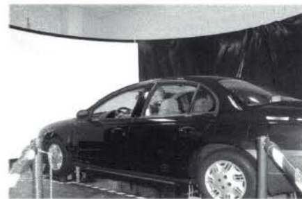
One of the laboratory tours featured the Highway Driving Simulator shown here. FHWA uses the simulator to test driver responses to various roadway situations and traffic control devices, such as collision avoidance systems.
