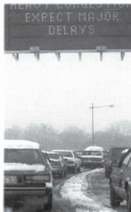
Variable message signs, like the one shown above, can alert drivers about congestion during adverse weather events, such as snowstorms, by providing real-time information.
