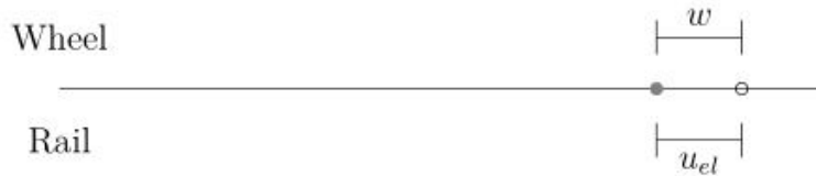
Figure 30. Situation 1: A wheel particle is displaced with respect to the rail by creepage. Initially, this rigid shift w is so low that it can be accommodated easily by elastic displacement.
