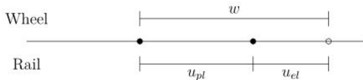
Figure 33. Situation 4: The creep is chosen such that the traction due to elastic deformation and plastic deformation adds up to exactly the traction bound: g = \mu p_n .
