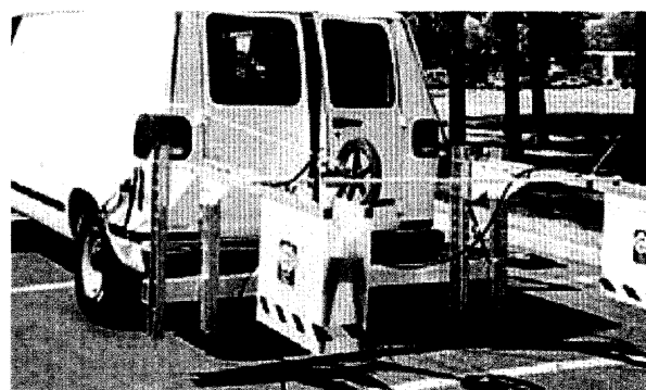
The advantage of using ground-penetrating radar systems, such as the one shown here, is the ability to collect continuous data at posted highway speeds. FHWA's new publication, Application of Geophysical Methods to Highway Related Problems , describes these systems and other geophysical methods.
