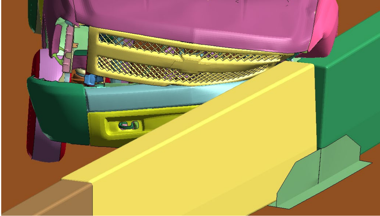
Figure 4.24 Concept No. 17 Snag Opportunity at Original Impact Point, 51 in. Upstream from Joint
