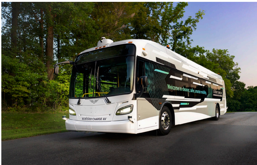
Figure 3-1 New Flyer Xcelsior AV transit bus equipped with an ADS from RRAI
