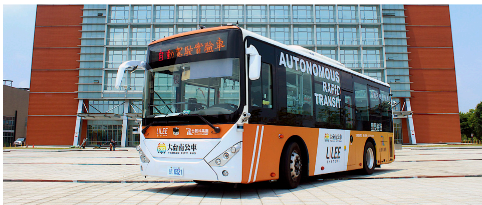
Figure 3-9 Transit bus equipped with an ADS from LILEE
