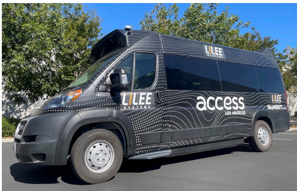
Figure 3-4 Dodge ProMaster bus equipped with an ADS from LILEE
