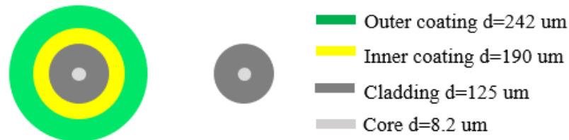
Figure 3.1 Optical fiber cross-sections before and after burning off outer and inner coatings
