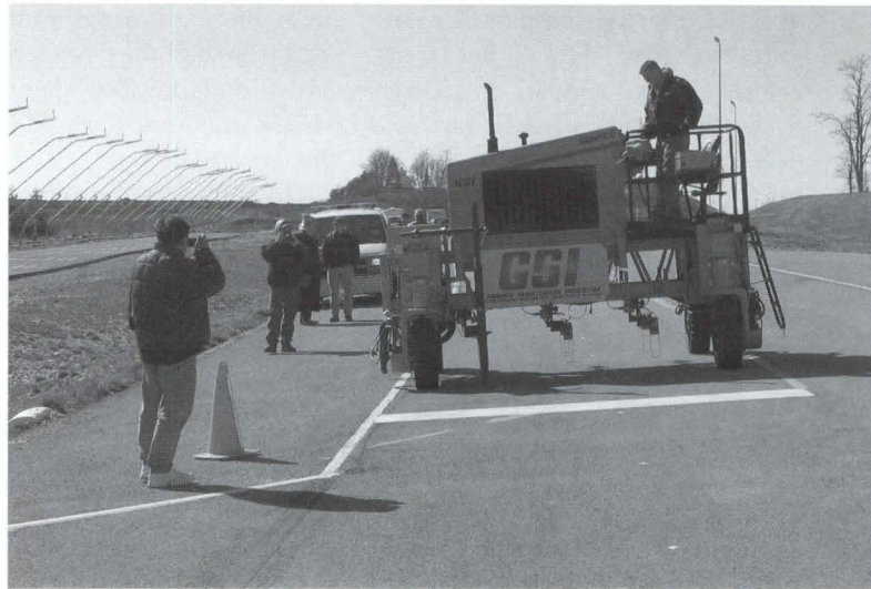
The GSI® profiler uses sonic technology to measure the pavement.
