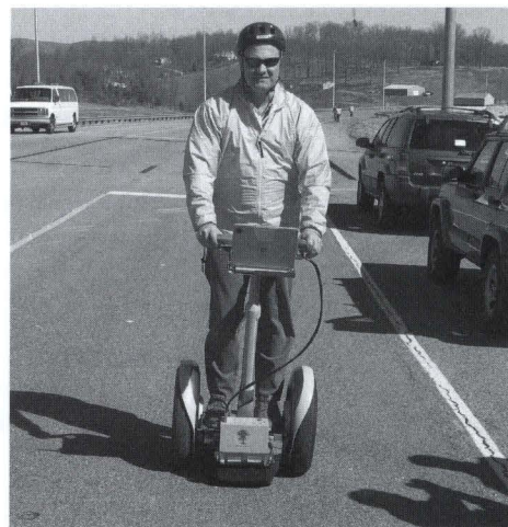
FHWA's ultra-light profiler was built using the Segway™ Human Transporter.
