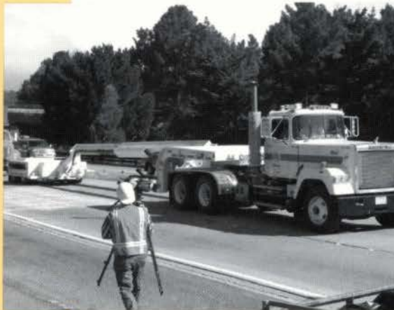
The Balsi Beam acts as a rigid obstacle to deflect traffic away from maintenance workers. A patent for the device is pending.
