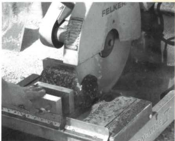
Top: The Superpave Performance Tester is run in the mobile asphalt lab. Bottom: Superpave Performance Tester specimens are prepared using a clamped sawing device.
