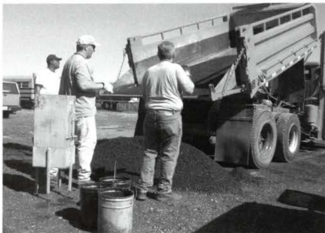
This photo shows the sampling and splitting of the asphalt mixture from Iowa's US 218 project for performance testing.
