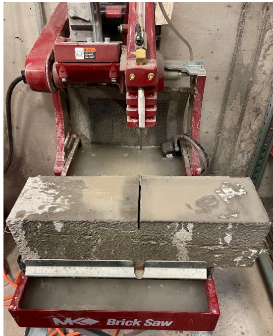
Figure 3.18 Notching the FRC Mini-Beams
