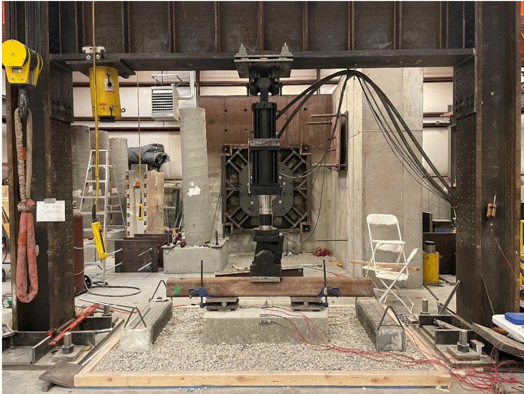
Figure 3.25 Testing Setup for Fatigue Analysis
