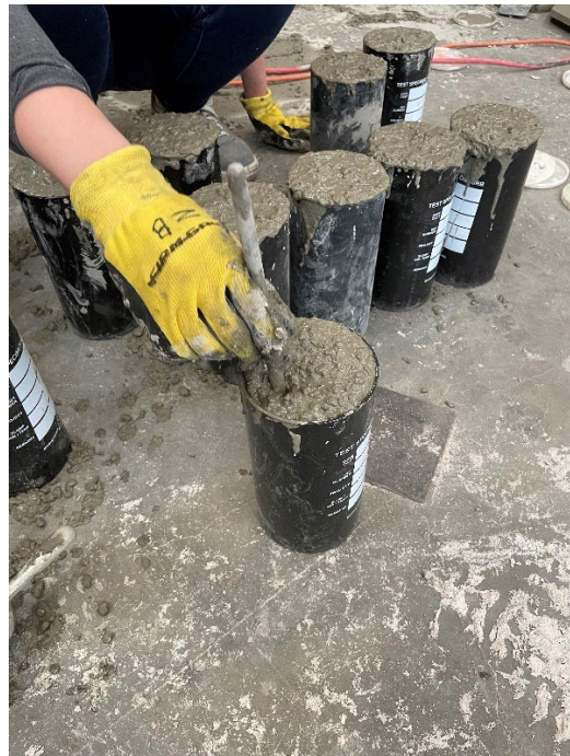
Figure B.5 Creating Concrete Cylinders
