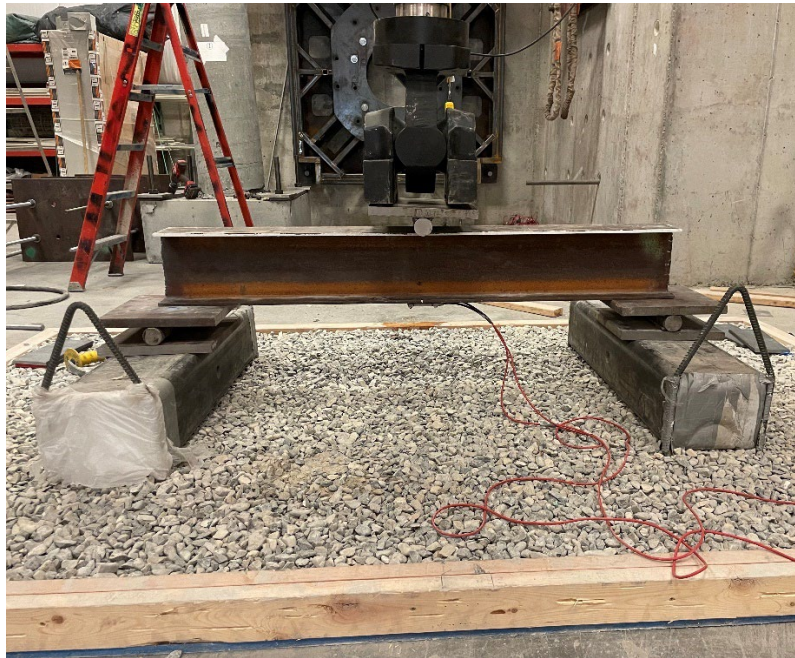
Figure 4.2 Strain Gauge Calibration Setup
