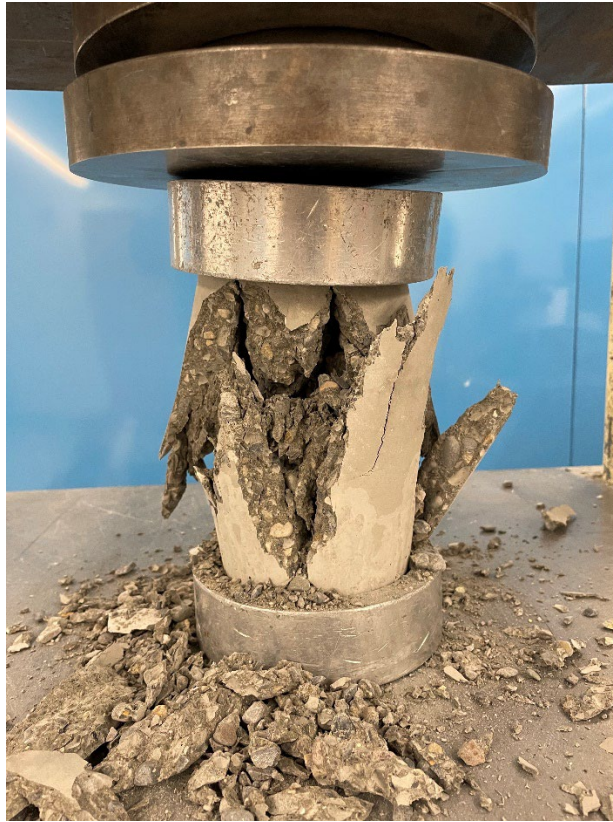
Figure 3.14 Typical Compression Testing Setup and Failed Cylinder
