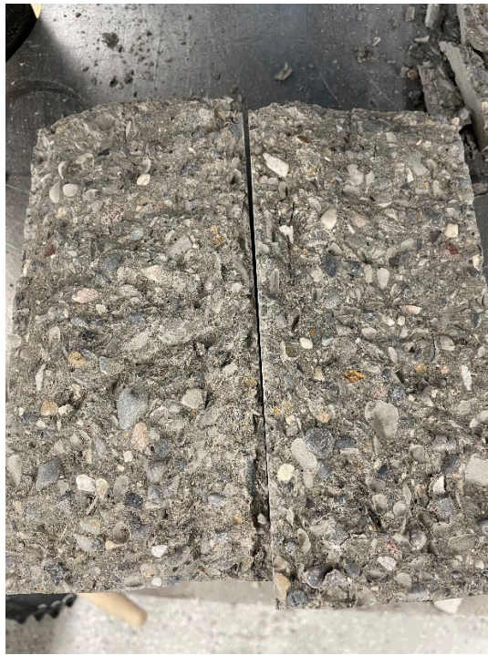
Figure 3.16 Plain Concrete Cylinder Failed During Tensile Test
