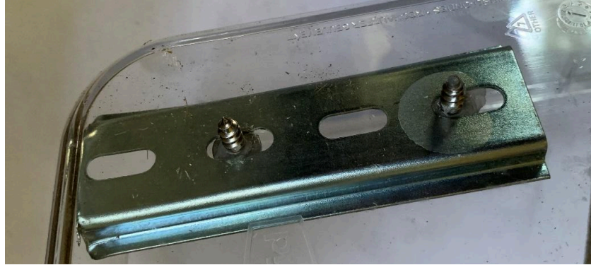
Image A11. Example of the silicon used to waterproof the holes, and the protrusion of the screws outside of the container.
