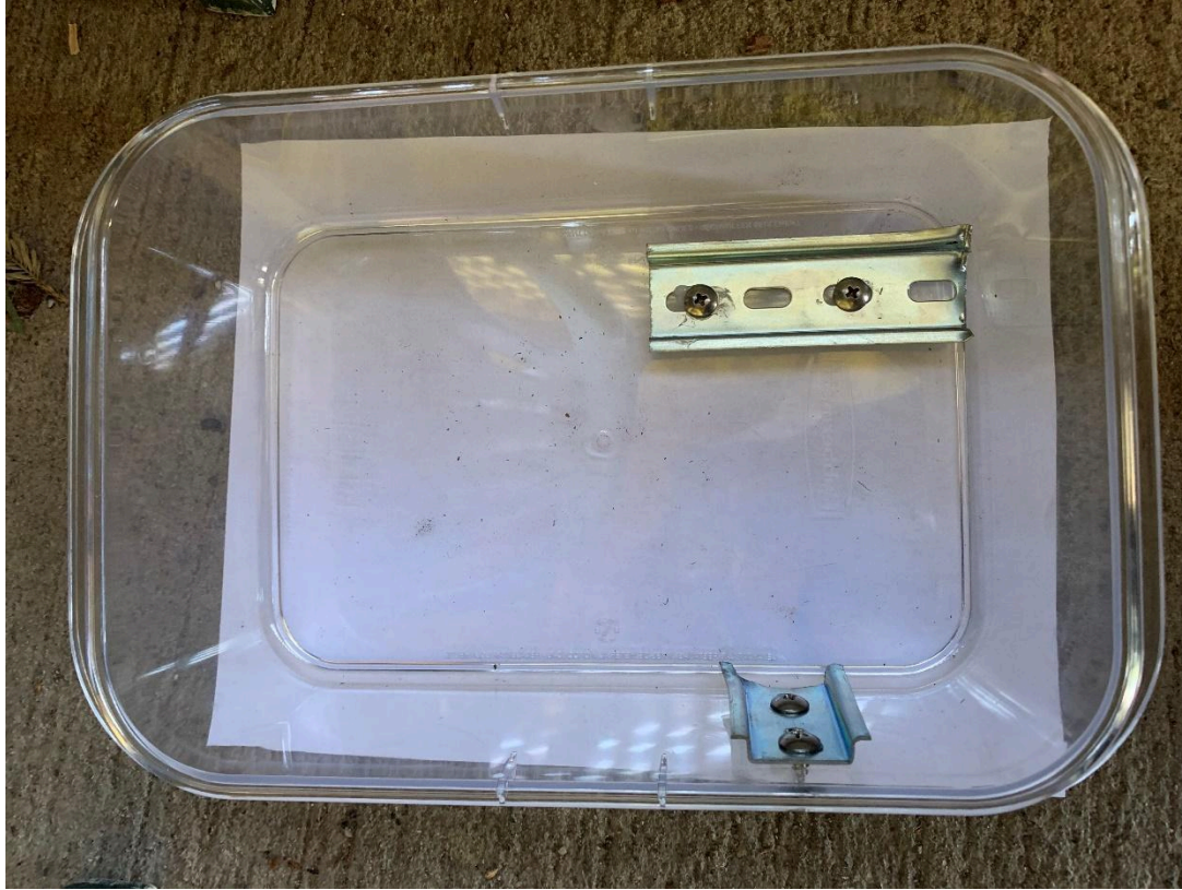
Image A10. Attachment points of the rail mounts for the Arduino and battery mounts.
