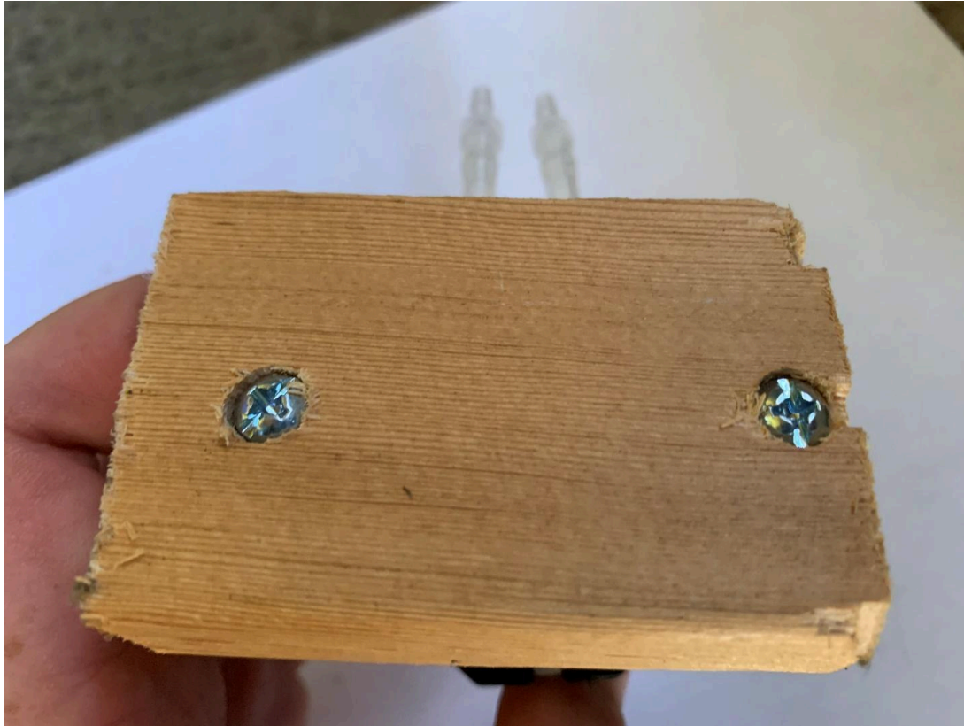
Image A6. Demonstration of the widened screw mount hole to allow for the mount to sit flatly against the Arduino container.
