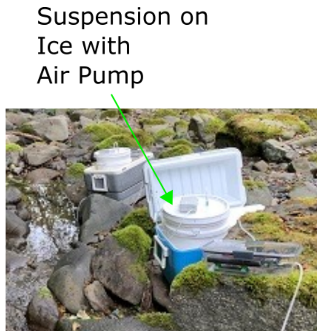
Figure 3. Representative deployment of two ADIDs in the field. Note the bucket containing FeDNA suspension was placed in a cooler on ice. The bucket was closed, and an air pump was attached to induce mixing.
