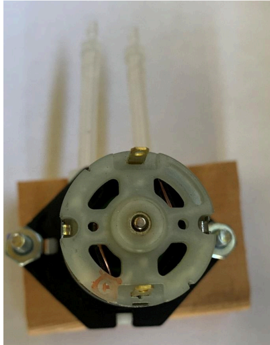
Image A5. Additional angle showing the mounting system on the peristaltic pump.
