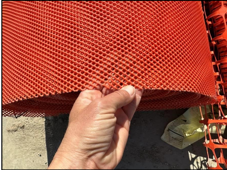
Figure 26. Fencing material with small mesh size to discourage chewing by kit foxes. (Photo by E. Noel)
