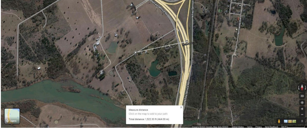
Original Photo: © 2022 Google® (see Acknowledgments page) Figure 2-24. Photo. Aerial top view: Horizontal Curve Radius 1,522.30 ft.
