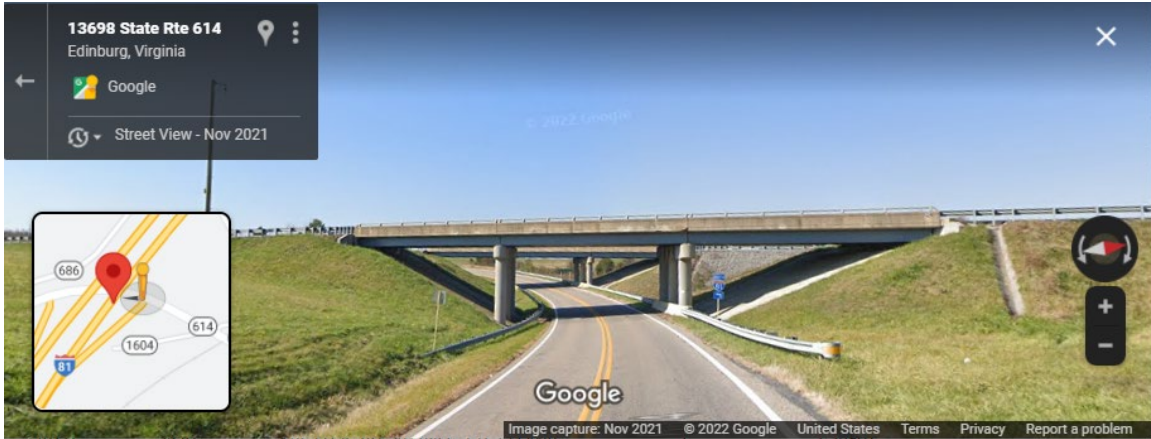
Figure 3-26. Photo. Example of Sharp curvature of driving lane below structure.
