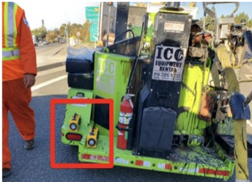
Figure 5.41 Placement of WAS Alarm Units on Rear of Equipment Vehicle
