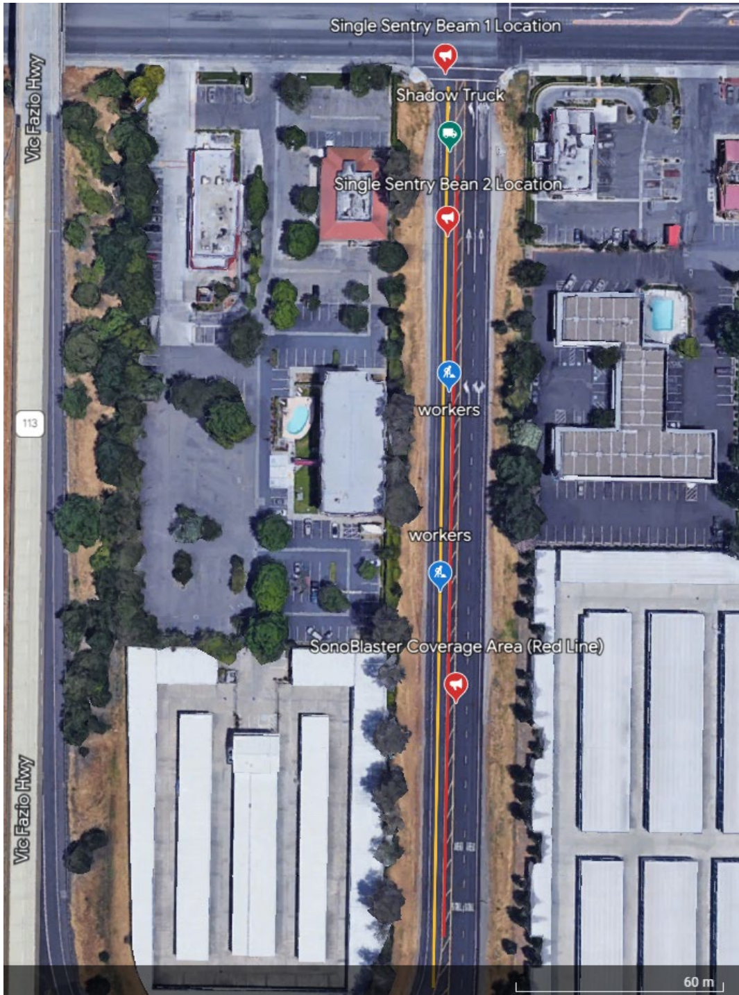
Figure 5.32 General Layout of Ramp Closure at CA Highway 113 and E Main St. (Source: Google Earth™)
