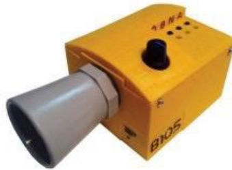
Figure A.1 Wireless Network System Sensor Node (Source: Martin et al., 2016)
