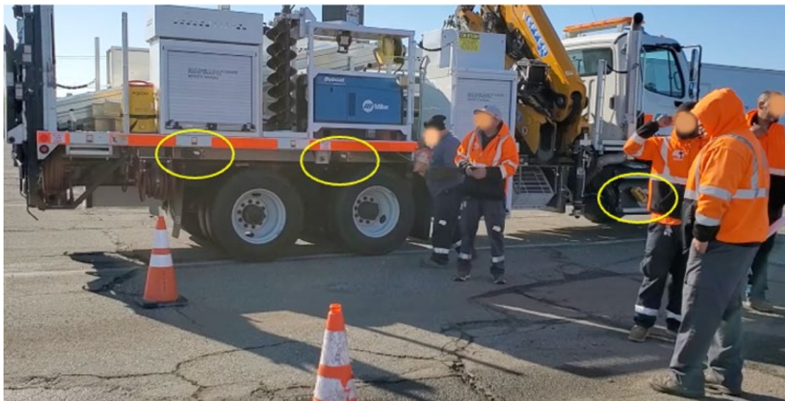
Figure 4.2 WAS Alarm Units’ Sound Test using Caltrans Generator Vehicle
