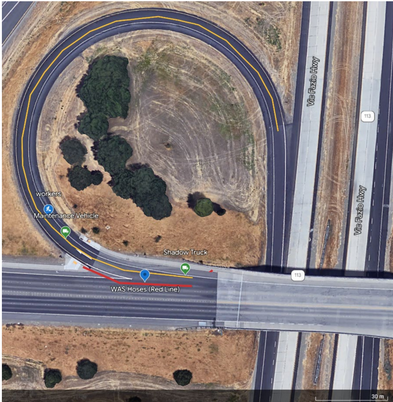
Figure 5.39 General Layout of Ramp Closure at CA Hwy 113 and E Gibson Rd. (Source: Google Earth™)
