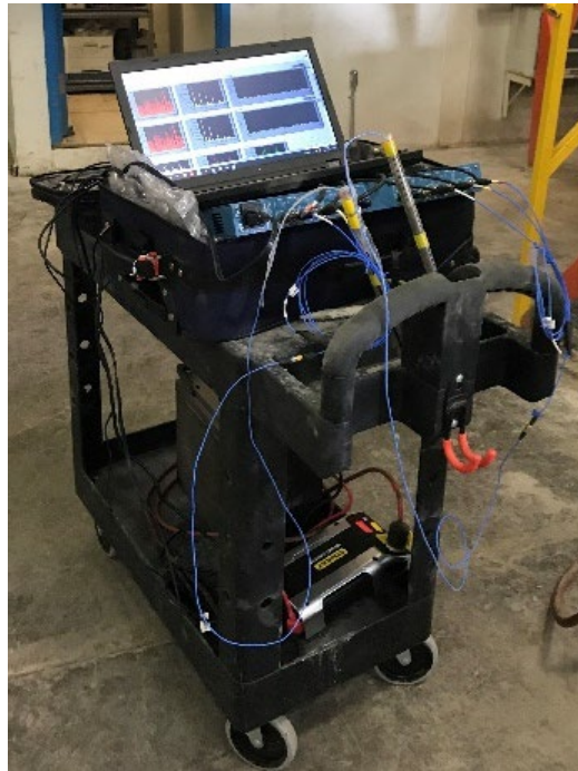
Figure 5. Acceleration measurement equipment cart
