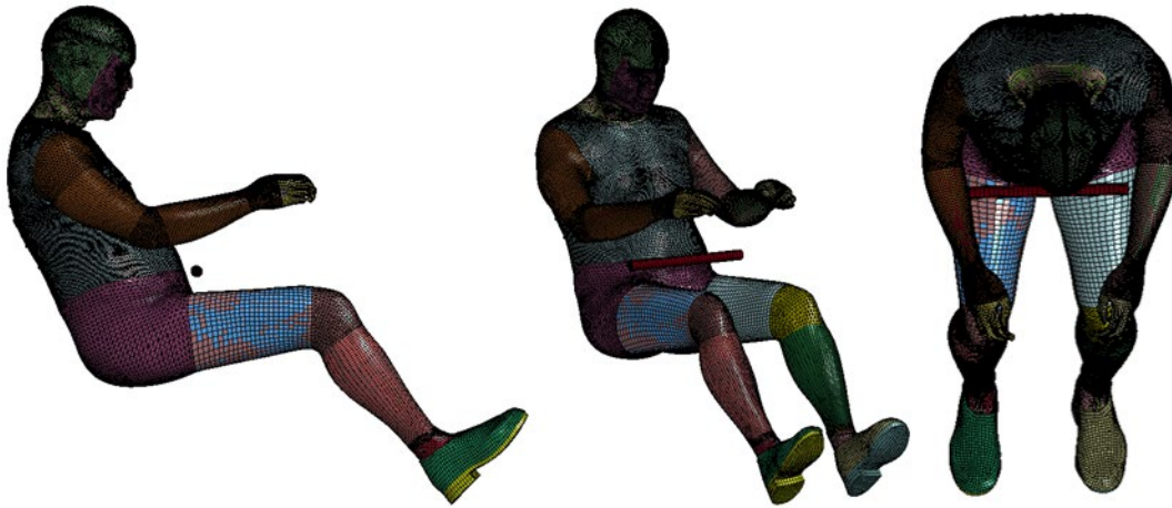
Figure 55. Set up of the abdominal bar impact with the GHBMC obesity model used in the belt pull tests
