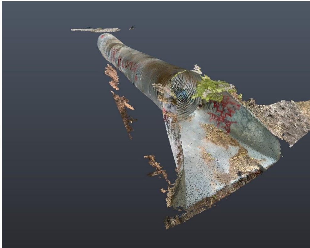
Figure 3.13.1 – Pocket LiDAR Point Cloud in Parley’s Historic Nature Park, Salt Lake County
