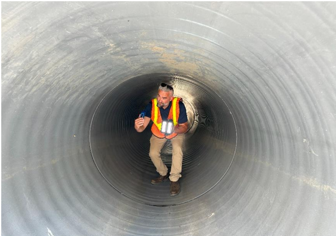
Figure 2.5.2 Photo of John Caya using iPhone to create 3D scan of Lisa Falls Cross Culvert, Little Cottonwood Canyon, August 7, 2023
