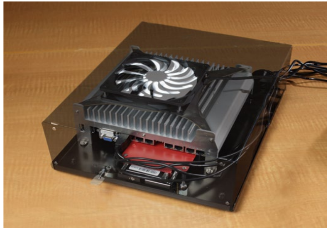
Figure 30. VTTI DAS main unit, mounted securely and inconspicuously
