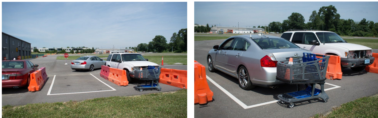
Figure 4. Position of automatically triggered shopping cart obstacle at the beginning and end of parking space backing trials
