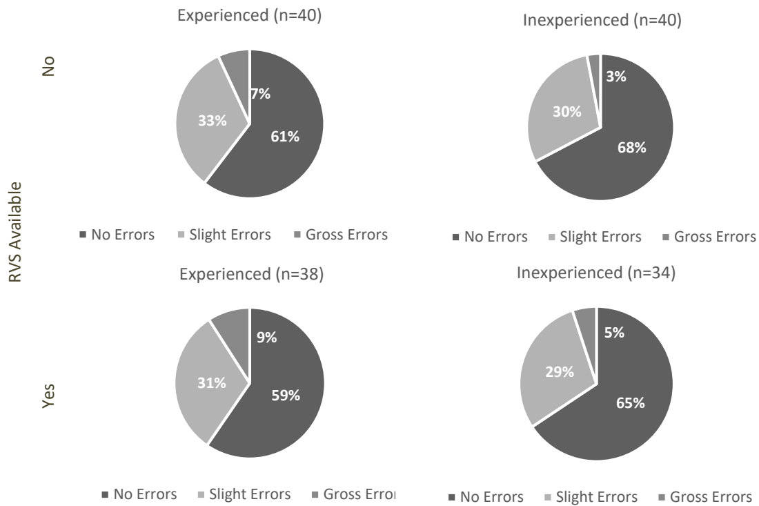
Figure 15. Overall long curved backing performance by RVS experience and availability (only including those participants who used RVS when available)
