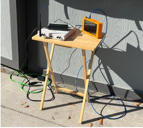
Figure 28. Photo. Field test setup (A SDR (the white box), a Raspberry Pi as a device hosting the SDR (the black box on the SDR), and a portable display (the orange box))
