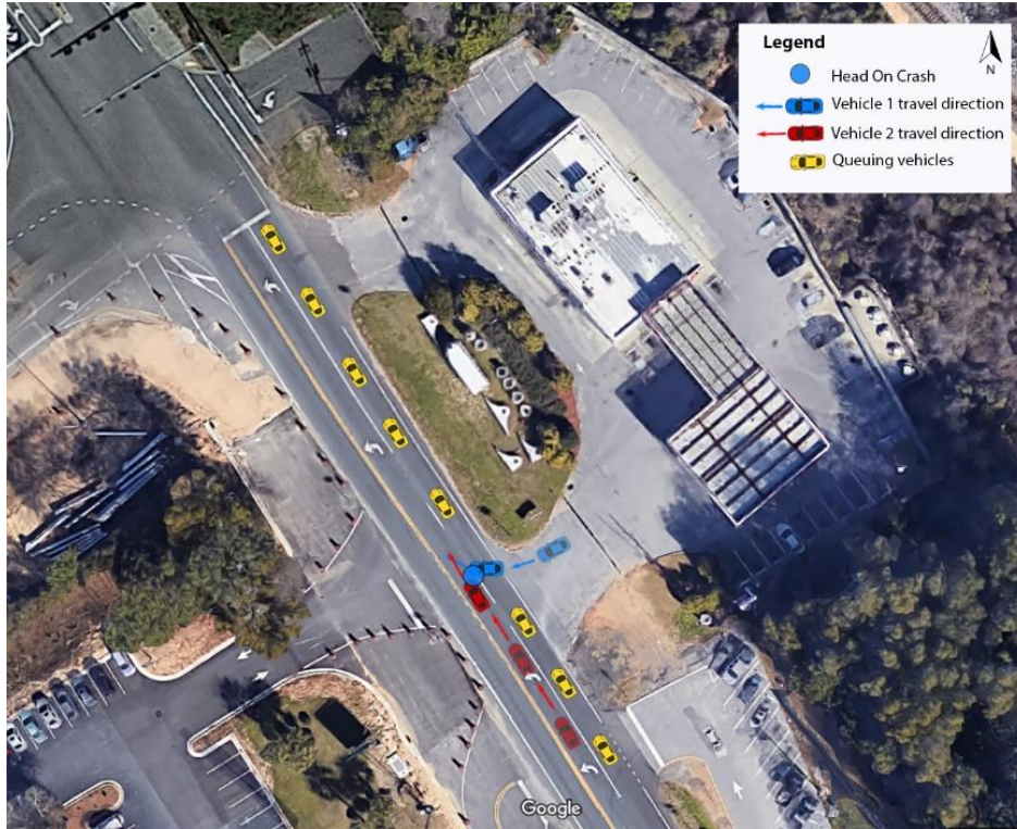
Figure 76. Right-turn out crashes at Scenic Highway at I-10 Interchange commercial plaza.
