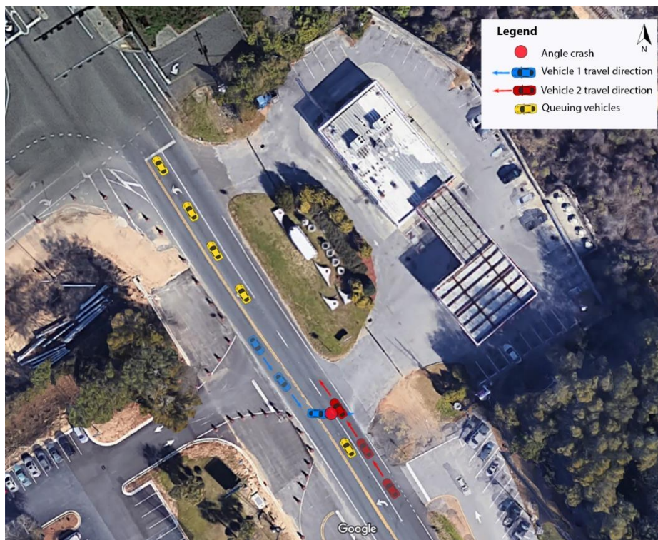
Figure 75. Left-turn in crashes at Scenic Highway at I-10 Interchange commercial plaza prior to median.
