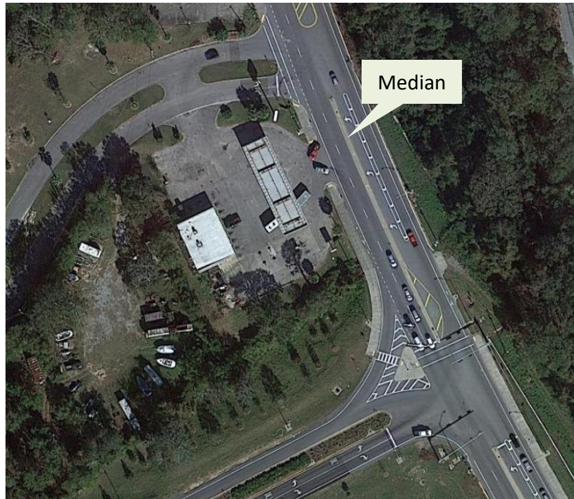
Figure 73. Commercial access and on-ramp design north of interchange following reconstruction.
