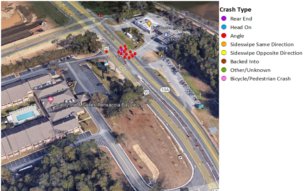
Figure 74. Configuration of access and crashes south of the Scenic Highway at I-10 interchange.
