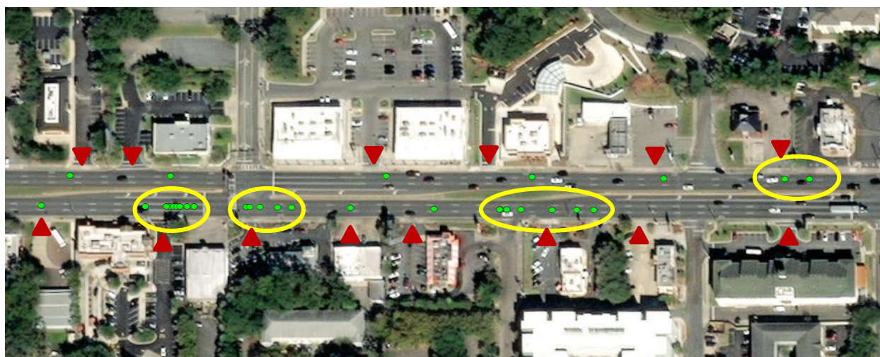
Figure 22. Example of crash clusters and crash assignment to corridor driveways.
