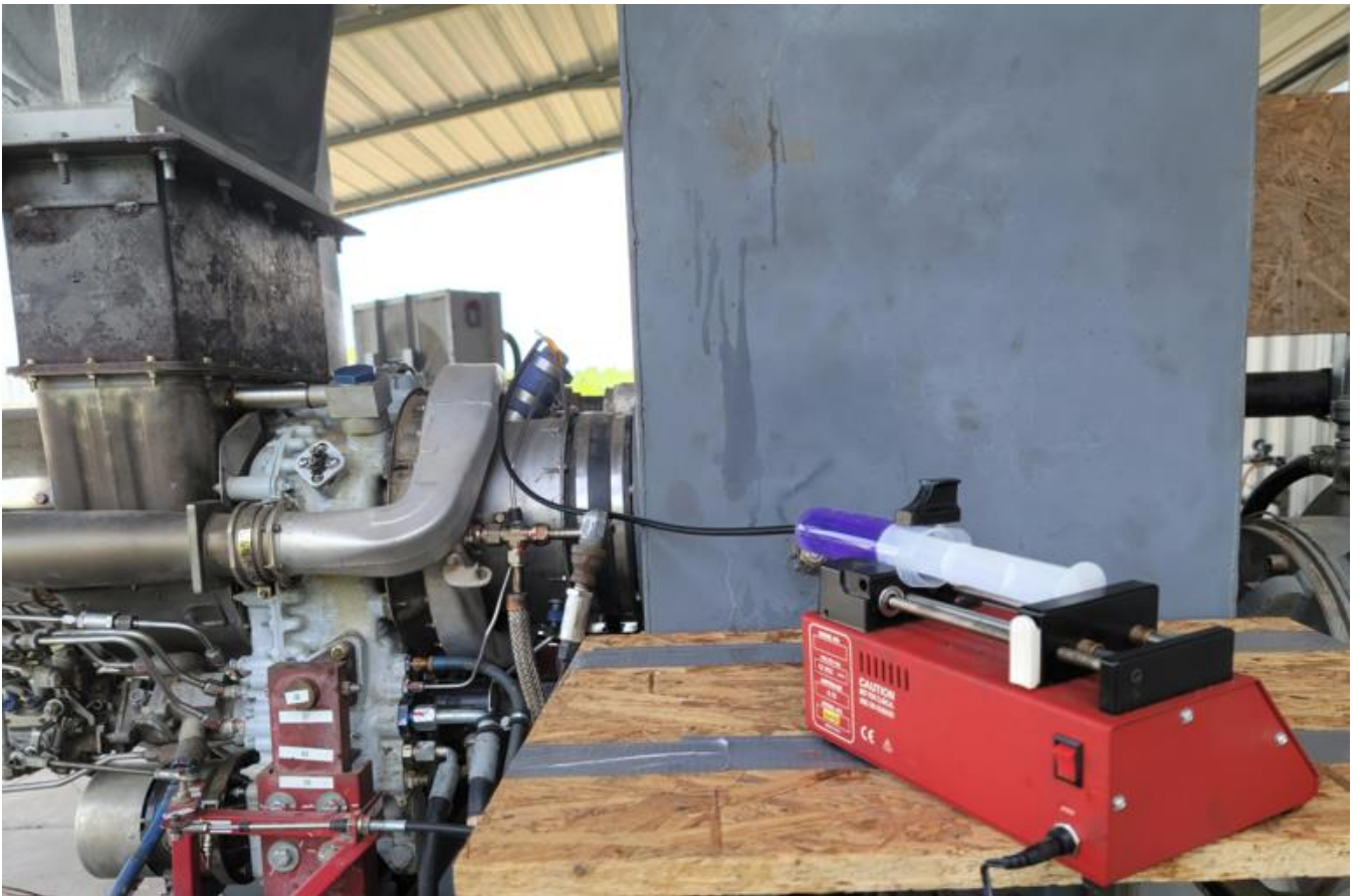
Figure 10. Contaminant injection syringe pump
