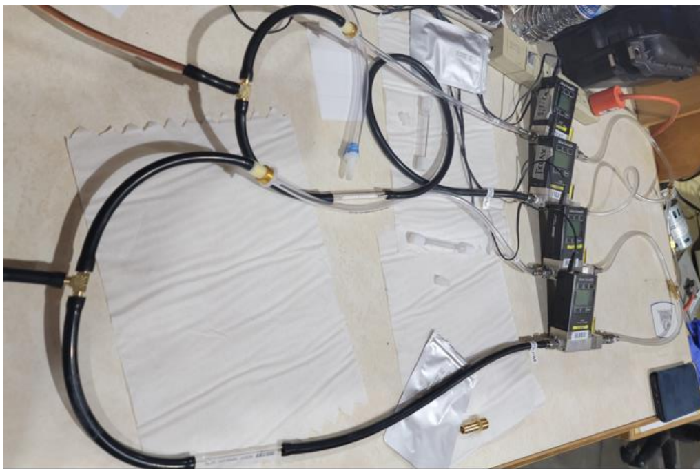
Figure 25. Alicat mass flow controllers with DNP and Tenax thermal desorption tubes
