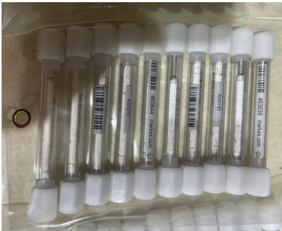
Figure 34. Single bed Tenax cartridges
