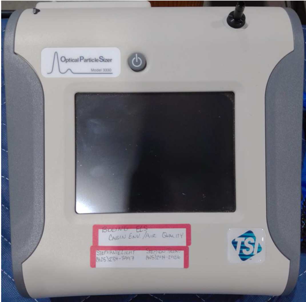
Figure I- 11. TSI 3330 Optical Particle Sizer
