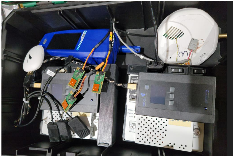
Figure 22. Chest for bleed sampling with diffusion sensors and low flow sensors instruments
