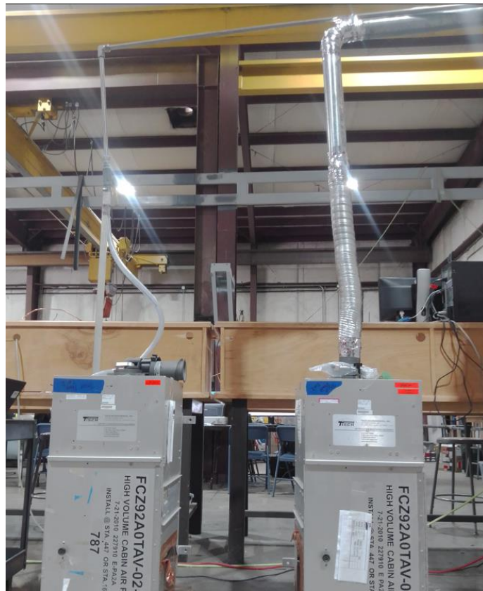
Figure 20. Ducting samples to atmospheric semi-volatile samplers
