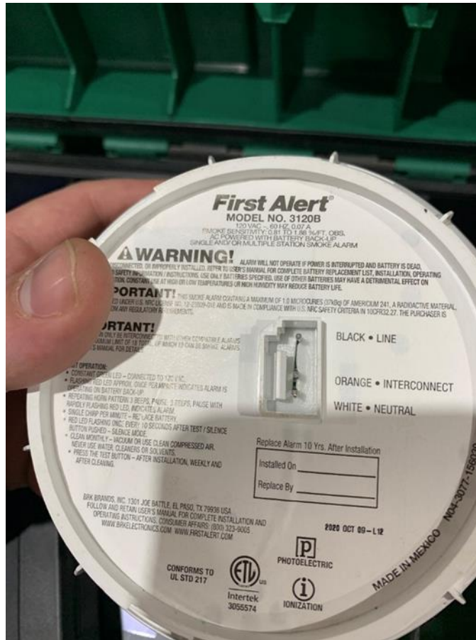
Figure I- 9. First Alert 3120B smoke detector
