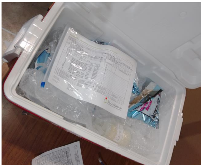
Figure 28. Ice chest and blue ice to maintain sample media at low temperature in transit
