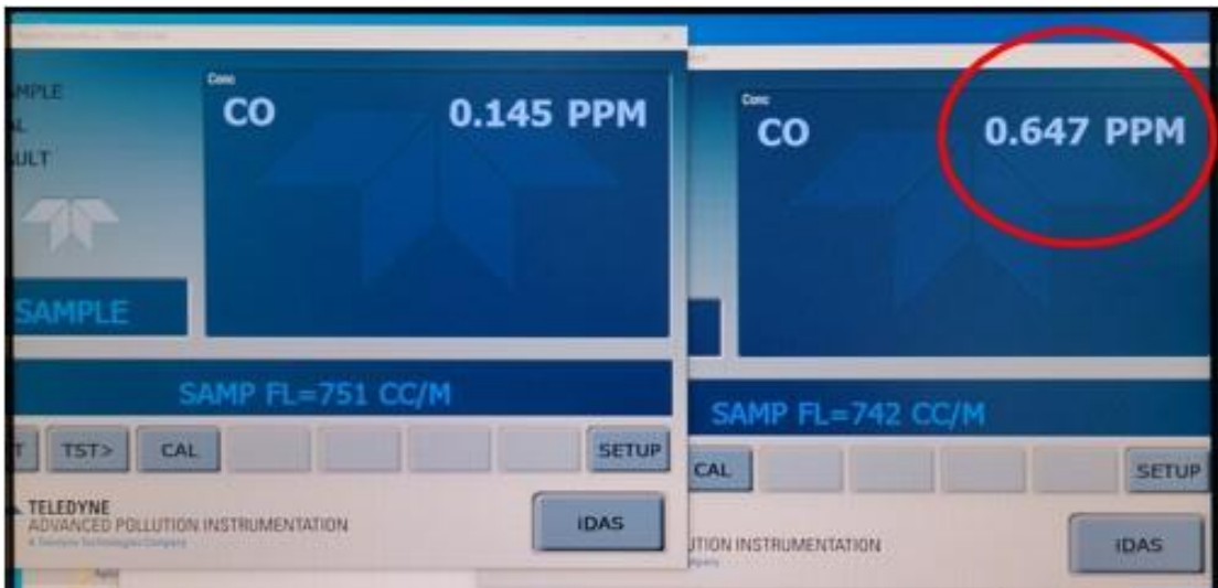
Figure 58. 0.6 ppbV response of Teledyne 300e CO analyzer to warming bleed air
