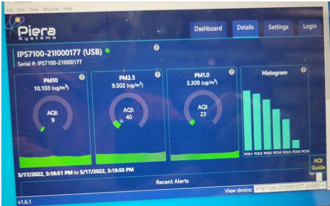
Figure I- 12. Piera Systems IPS-7100 Particle Sensor
