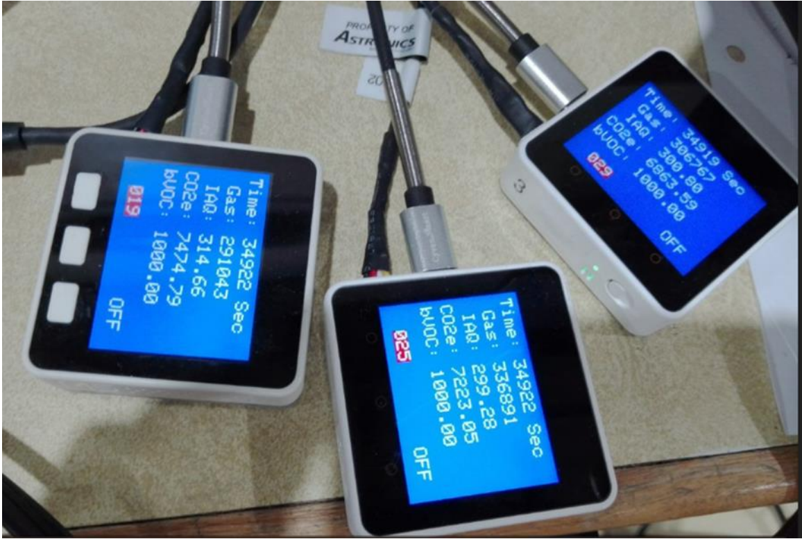
Figure I- 19. Astronics metal oxide sensors
