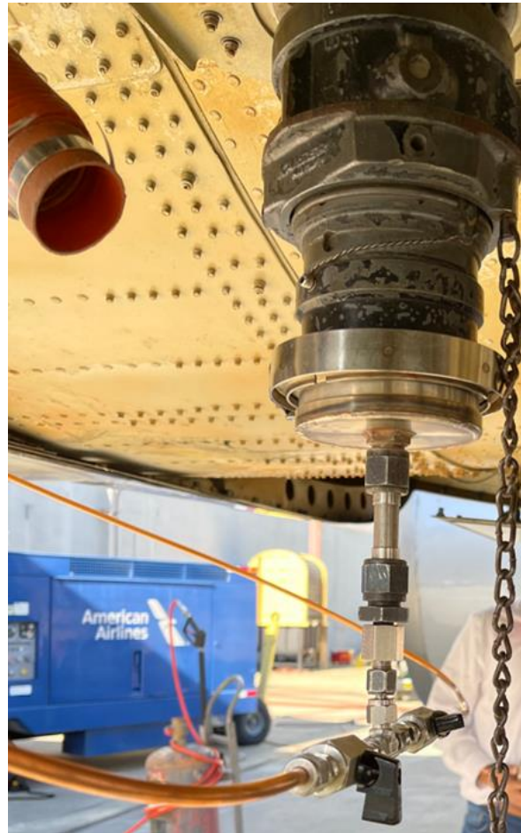
Figure 121. HP sampling with dedicated lines for two fluid types
