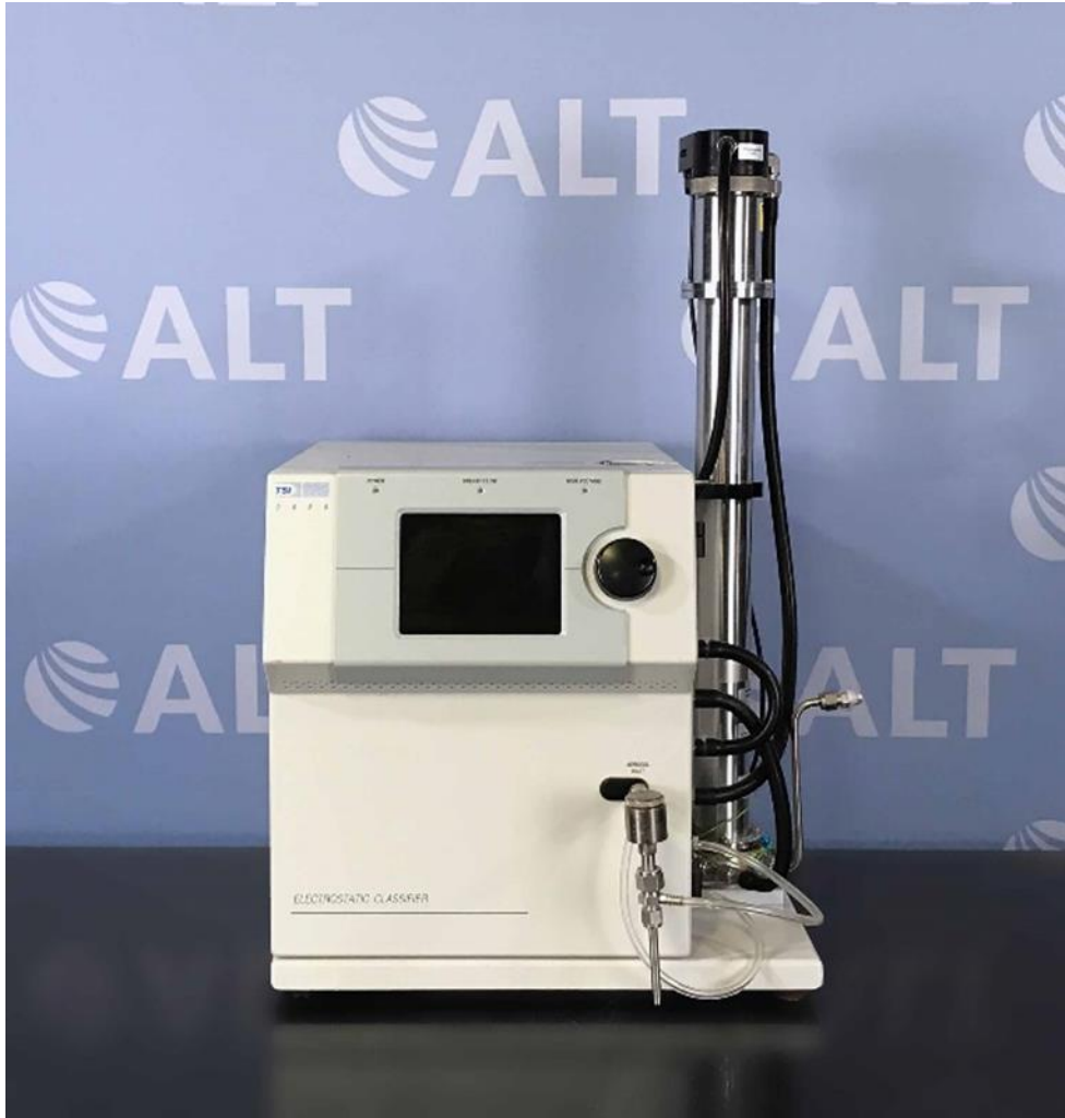
Figure I- 1. TSI 308000 electrostatic classifier
