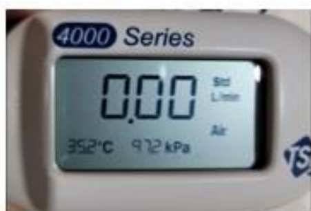
Figure 26. TSI Model 4000 flowmeter transfer standard for mass flow controllers (Photo courtesy of TSI Incorporated)
