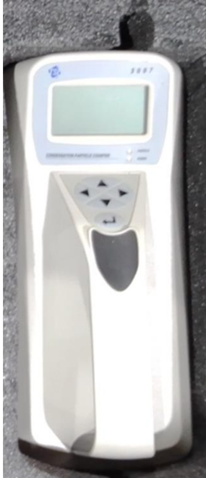
Figure I- 4. TSI 3007 handheld condensation particle counter
