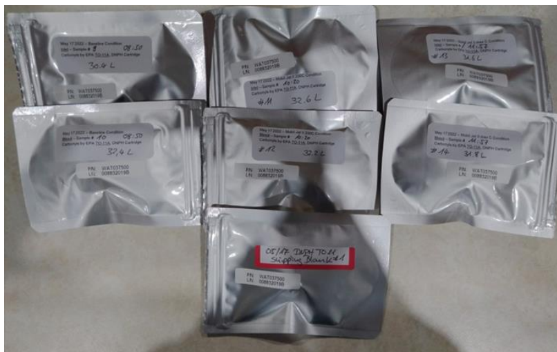
Figure 27. Waters PN WAT037500 DNPH cartridges without ozone scrubbers
