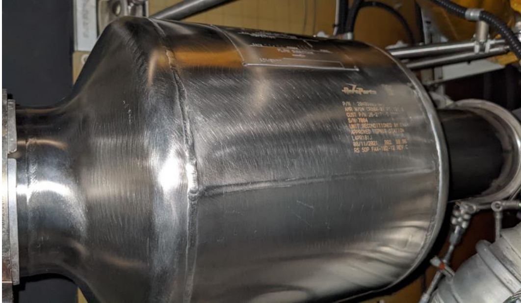
Figure 118. BASF OEM AeroCoat® VOC /Ozone converter installed on the right side of the aircraft under test
