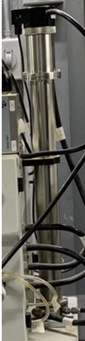
Figure I- 2. TSI 308701 X-Ray particle neutralizer
