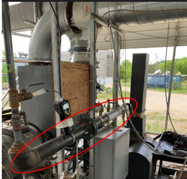
Figure 14. Bleed air sample line - bleed air heat exchanger to stainless steel sample line
