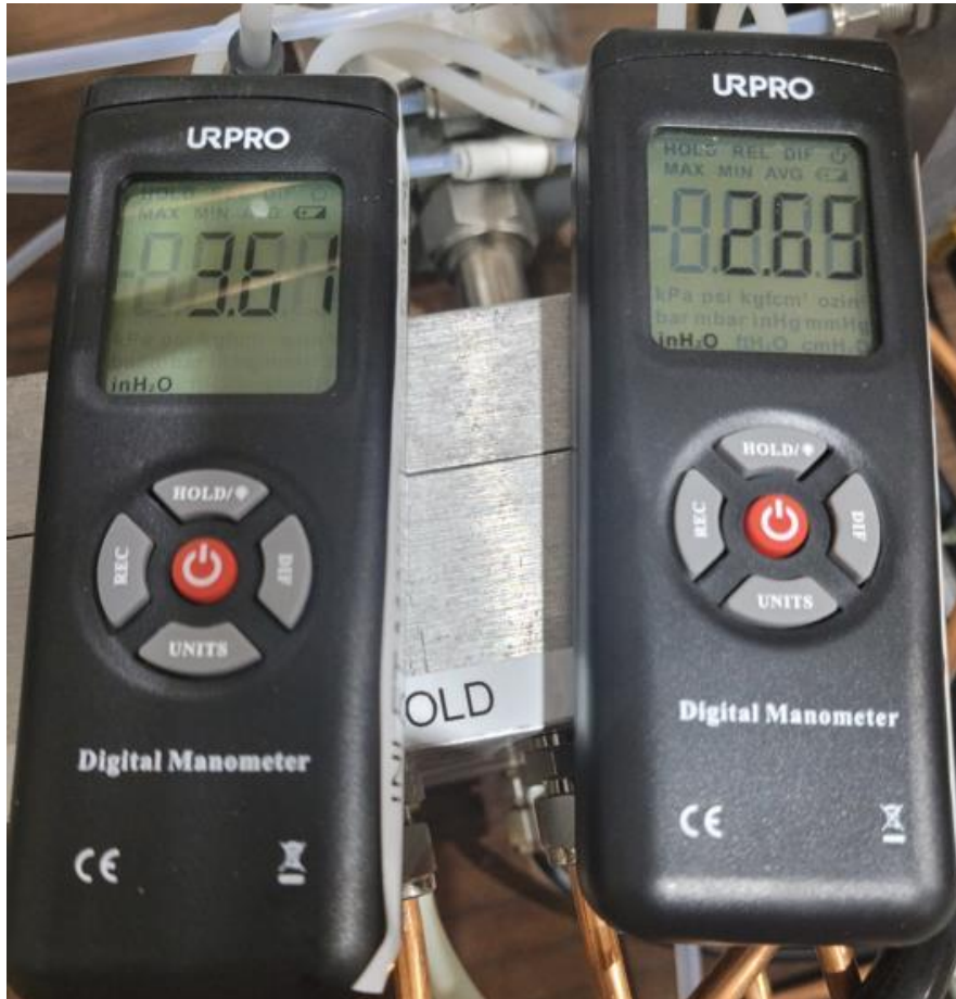
Figure 18. URPRO digital manometers to monitor inlet and bleed sample manifolds
