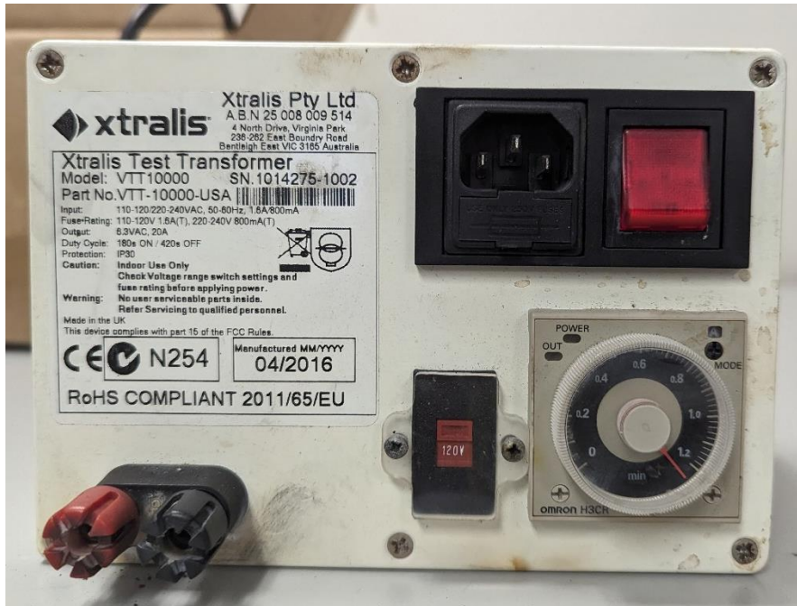
Figure 6.2 Xtralis Test Transformer used for cable failure tests
