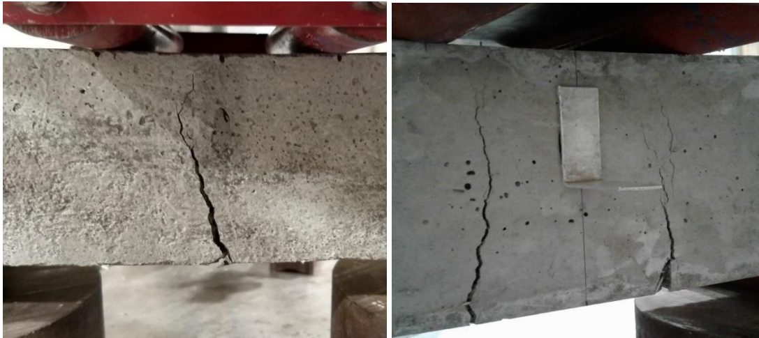
Figure 4. Close-up view of single (left) and double (right) crack pattern failure
