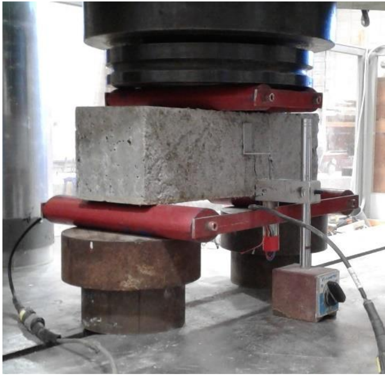
Figure 2. Flexural test setup: main dimensions (top) and full configuration (bottom)
