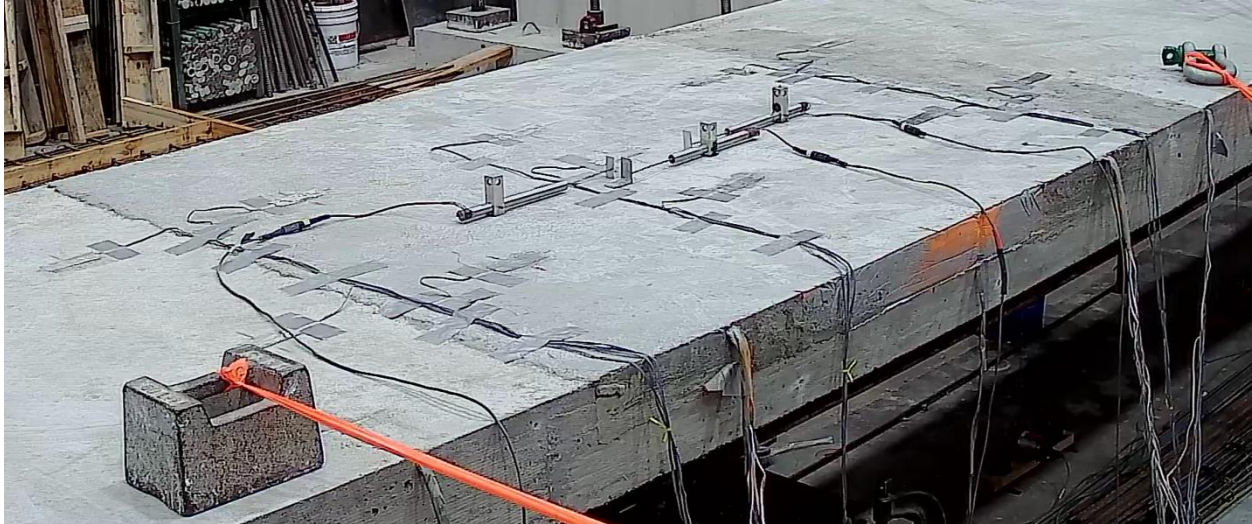
Figure 17. DCDTs and surface strain gauges
