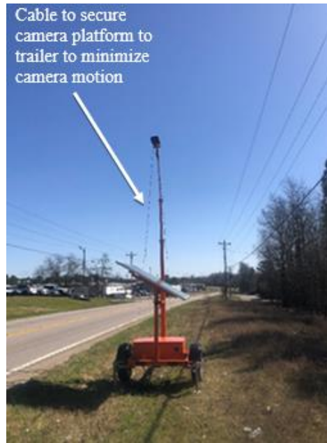
Figure 4: Thermal camera and trailer at a data collection site
