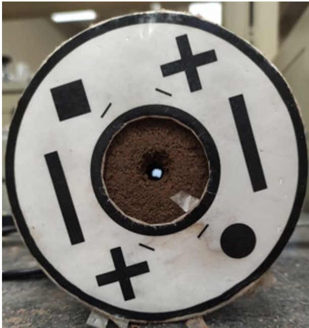
Figure 10. Calibration marker on the downstream hole of an eroded sample.
