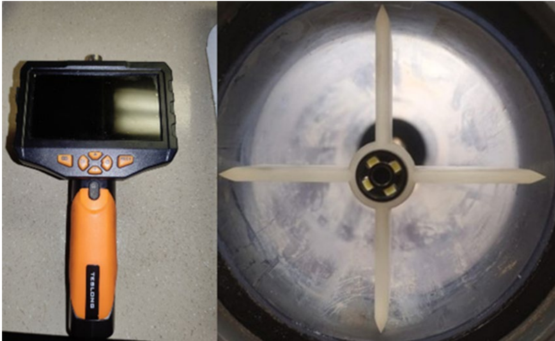
Figure 11.(a) Viewing screen and operating controller, (b) Camera shown with holder and 3D printed support
