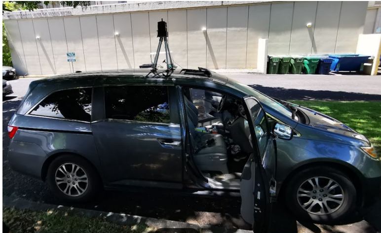
Fig. 3. The MCS system that shows the 360° degree camera mounted on top of a vehicle.
