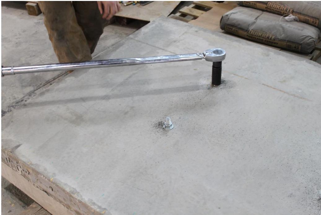
Figure 3.9 Researcher tightening the proprietary anchor to manufacturer's specifications.
