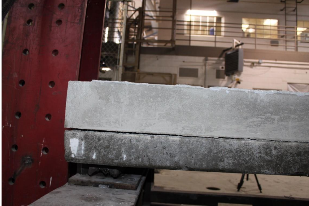
Figure 5.3 Delamination at northwest corner of control specimen at 2.4 in. of displacement.
