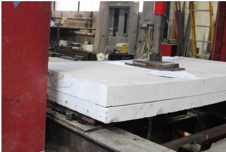
Figure 5.31 Delamination of CIP and PC decks at 1.6 in. of applied displacement. (Location: southeast).
