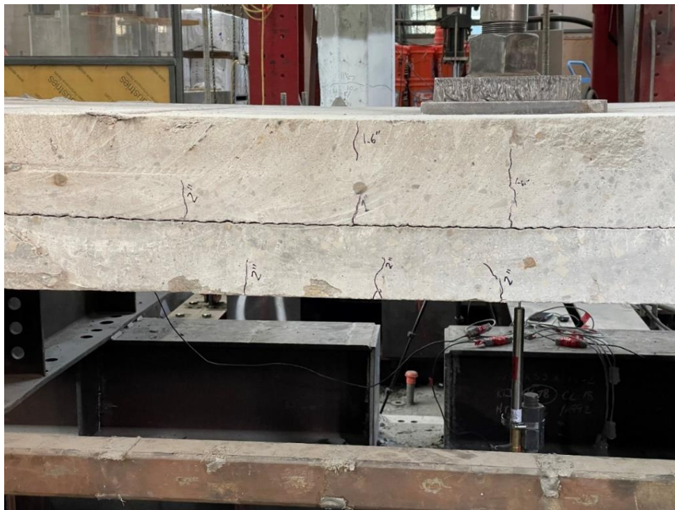
Figure 5.19 CFRP retrofit deck delamination at 2.0-in. displacement (Location: east, mid-span)
