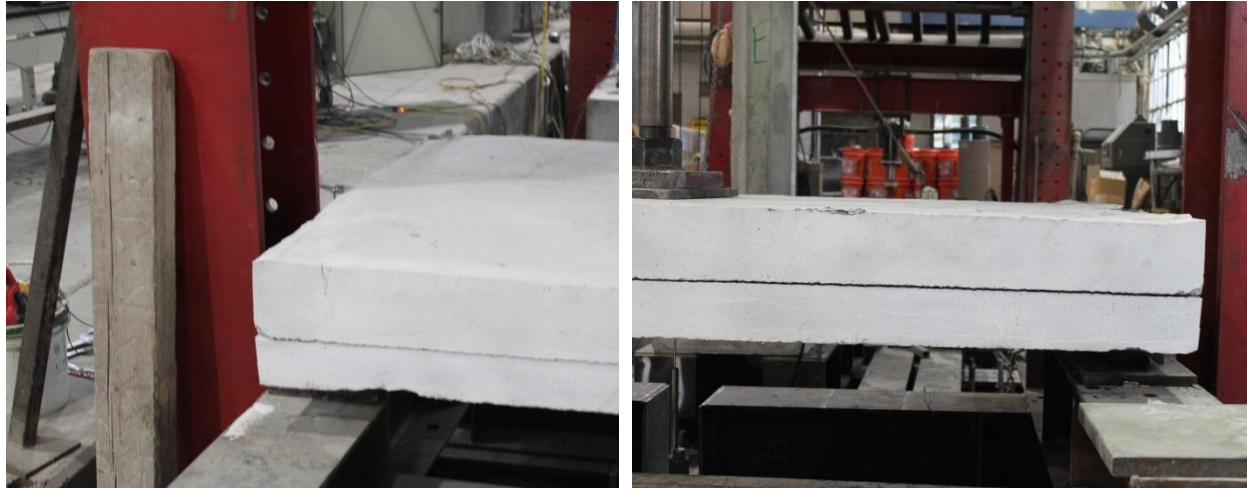
Figure 5.12 Shear anchor retrofit deck panel initial delamination. (Location: left; southeast, right; northeast)
