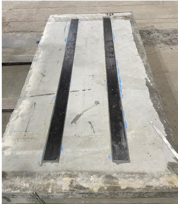
Figure 3.13 Underside of test panel with CFRP strip installed.
