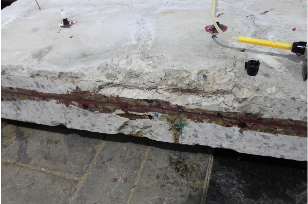
Figure 6.11 Salvaged panel being injected with epoxy.
