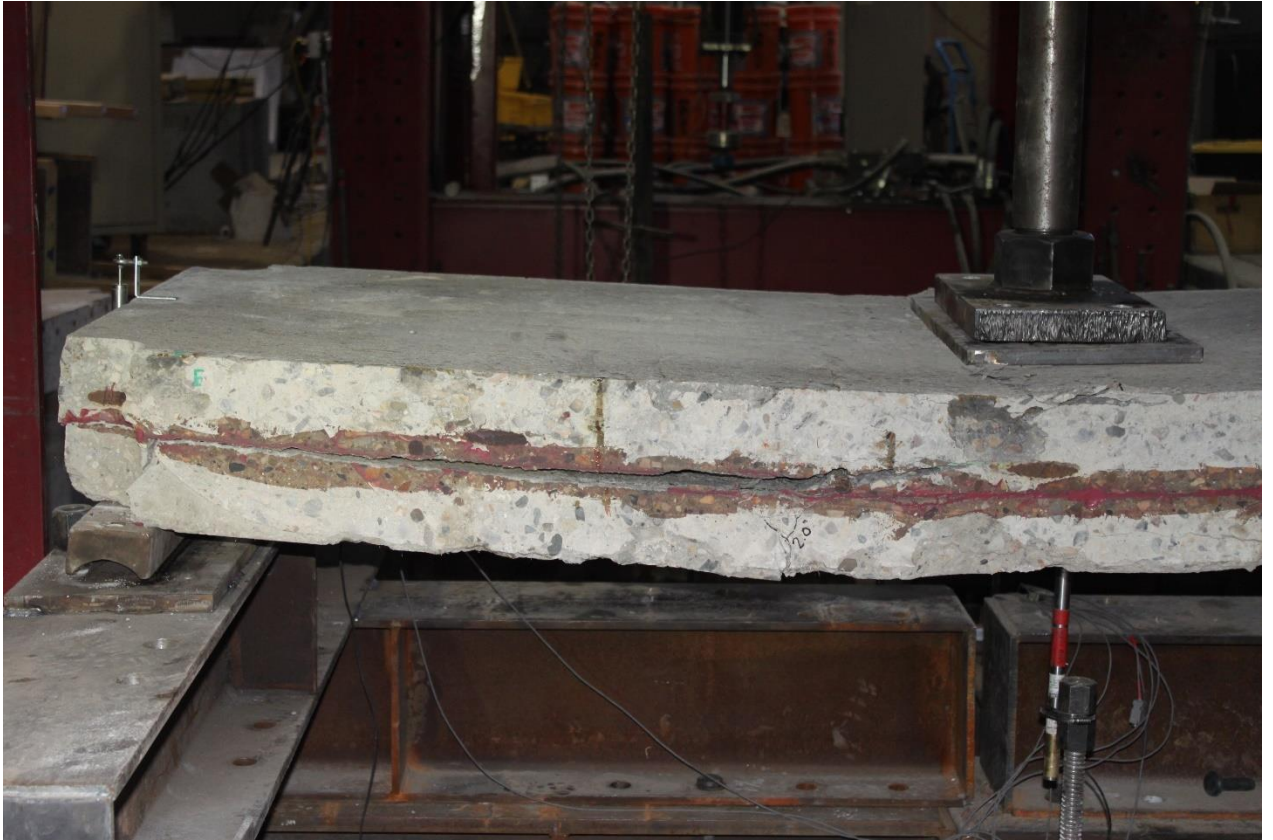
Figure 6.12 Epoxy bond failure of P-B after 2.5 in. of applied displacement. (Location: southeast)
