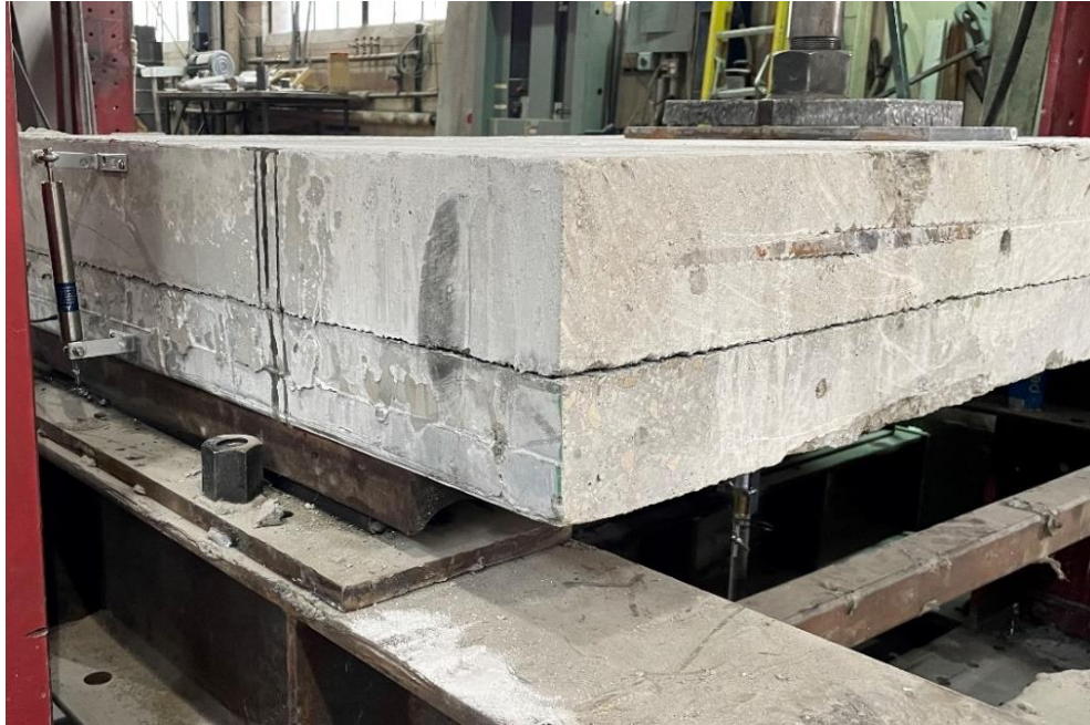
Figure 5.17 CFRP retrofit deck panel initial delamination prior to testing. (Location: southeast corner)
