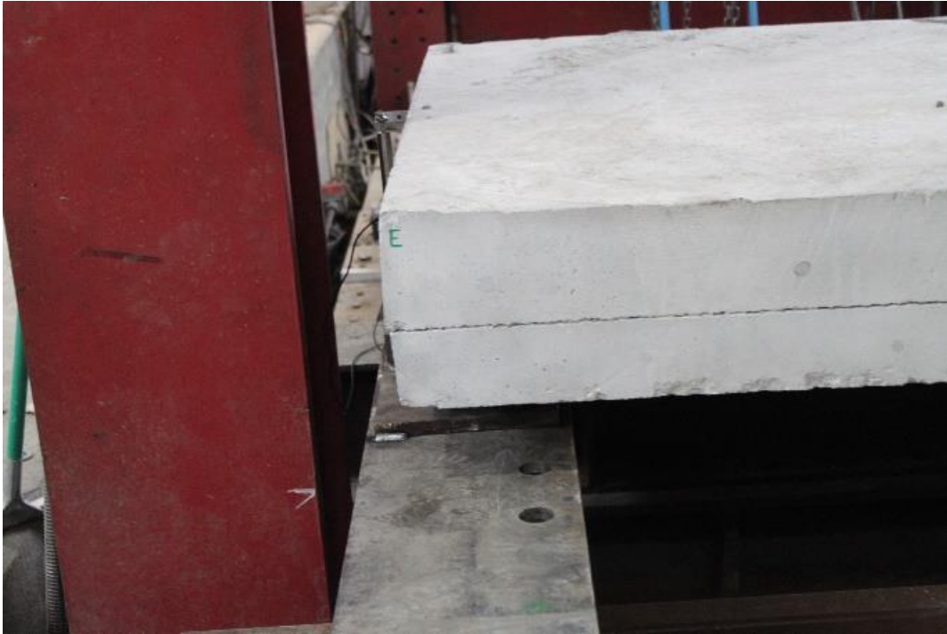
Figure 5.25 CIP and precast deck panel at 2.0 in. of displacement. (Location: southeast).
