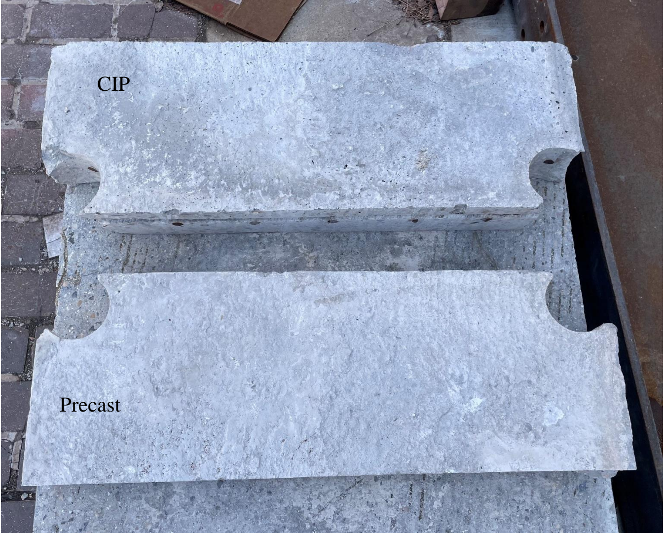
Figure 6.5 Cut section of P-B separated exposing mating interface between panels.
