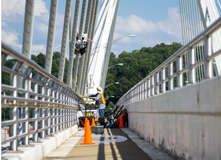
Figure 92. Photo. The test setup for the Pomeroy-Mason Bridge on the sidewalk.
