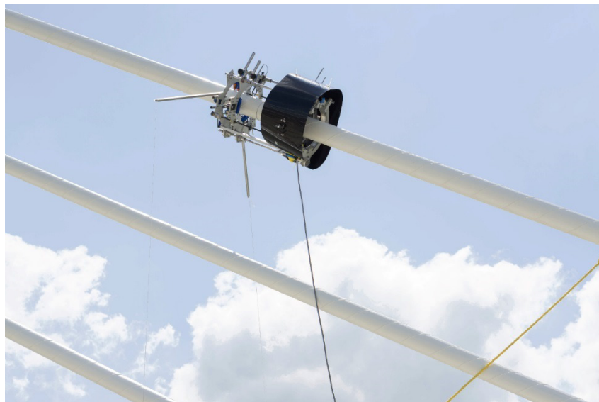
Figure 46. Photo. The robot climbing a cable on the Ironton-Russell Bridge.
