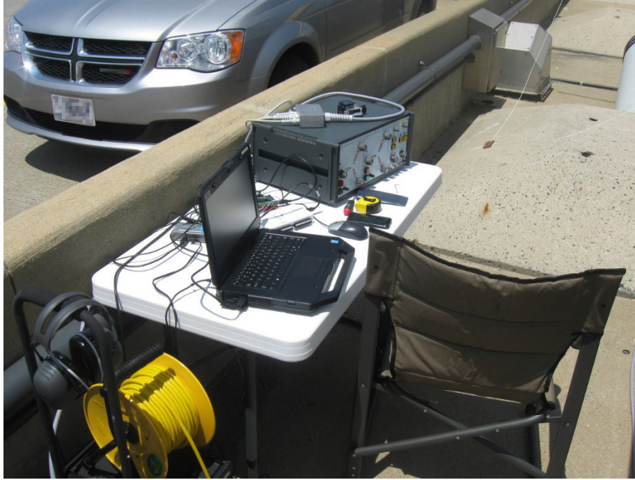
Figure 13. Photo. The laptop, DAQ module, and control unit.
