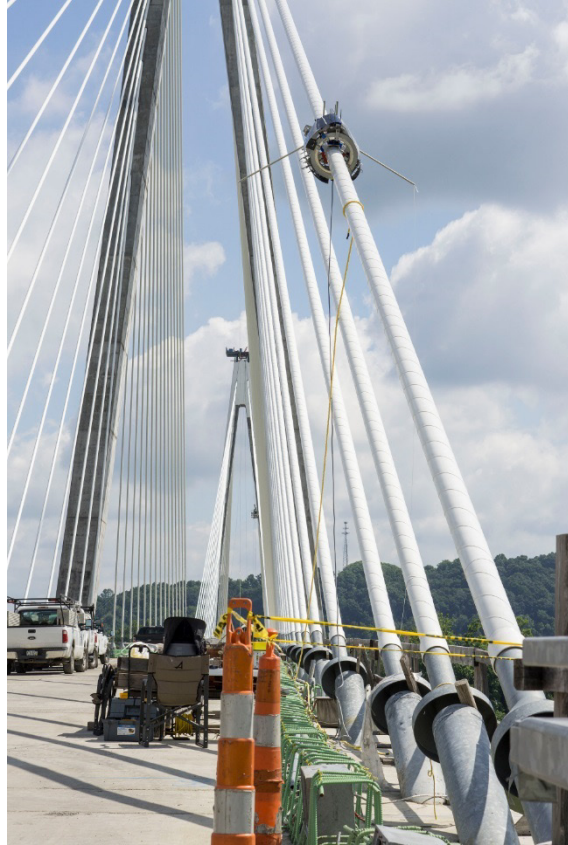
Figure 46. Photo. The robot climbing a cable on the Ironton-Russell Bridge.
