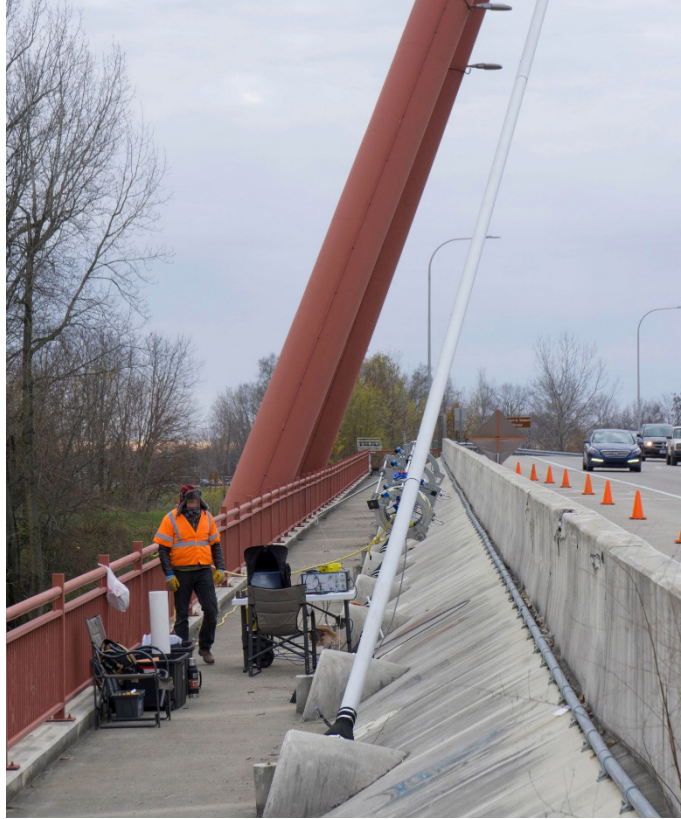
Figure 76. Photo. The robot climbing a cable from the Robert N. Stewart Bridge.
