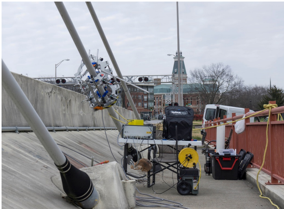
Figure 76. Photo. The robot climbing a cable from the Robert N. Stewart Bridge.
