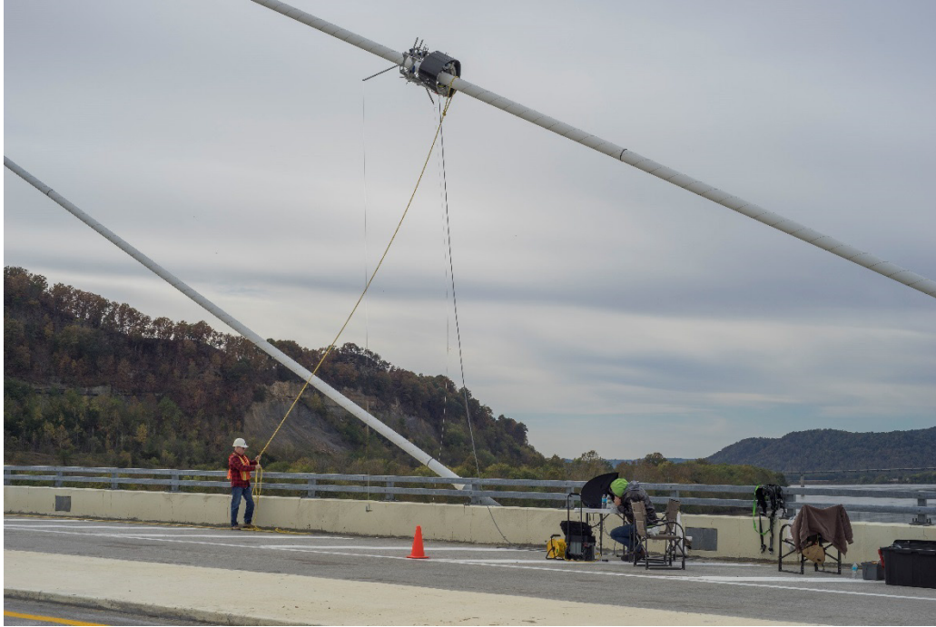
Figure 57. Photo. The robot climbing a cable at the U.S. Grant Bridge.
