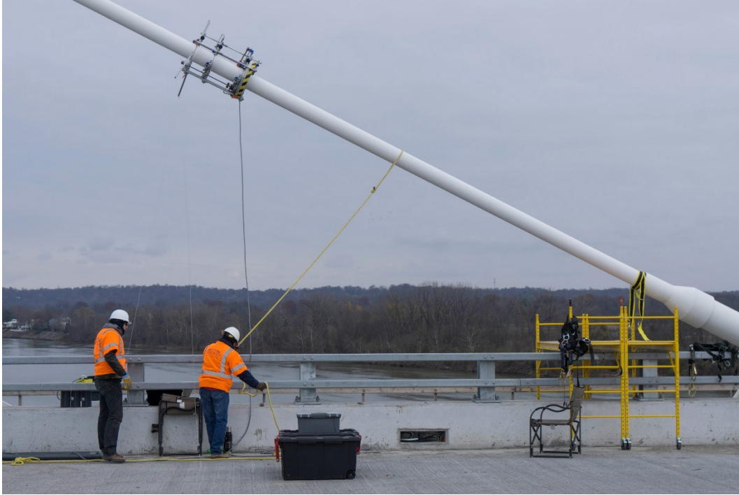
Figure 67. Photo. The test setup on the East End Bridge, including the scaffolding near the cable anchorage.
