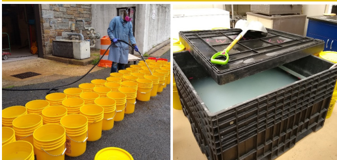
A. Photograph. 47 buckets needed to condition 141 concrete cylinder specimens in APS.
