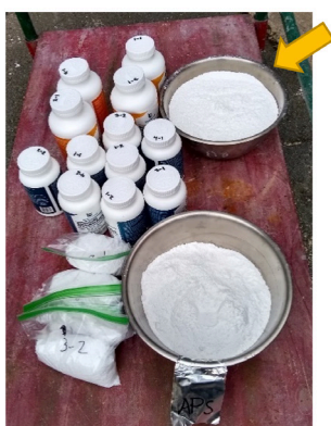
Figure 3. Photograph. Chemicals used to develop one tank of APS, along with the single bowl of Ca(OH) 2 needed to develop a tank of LW.
