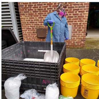
Figure 4. Photograph. Reactivity precautions that must be taken to develop large volumes of APS, including ice to reduce the temperature of the solution and a plastic shovel to stir without introducing metals to the solution.
