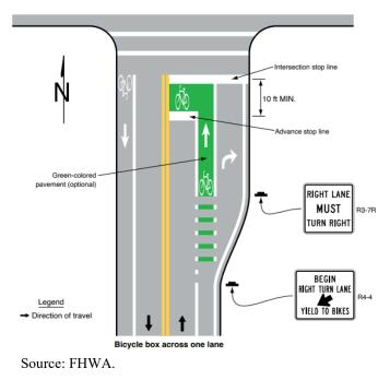
Figure 27. Photograph. Example of a bike box (FHWA 2023b).
