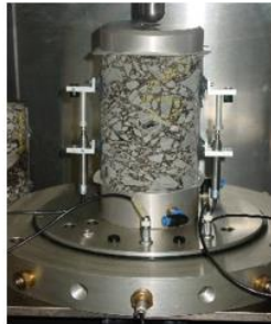
(c) Sample Setup for LTRC |E^*| test
